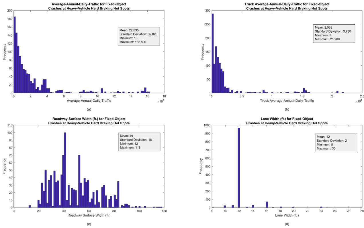
**Figure 3.17: (a) AADT, (b) HV-AADT, (c) Roadway Surface Width, and (d) Lane Width for Fixed-Object Crashes**
