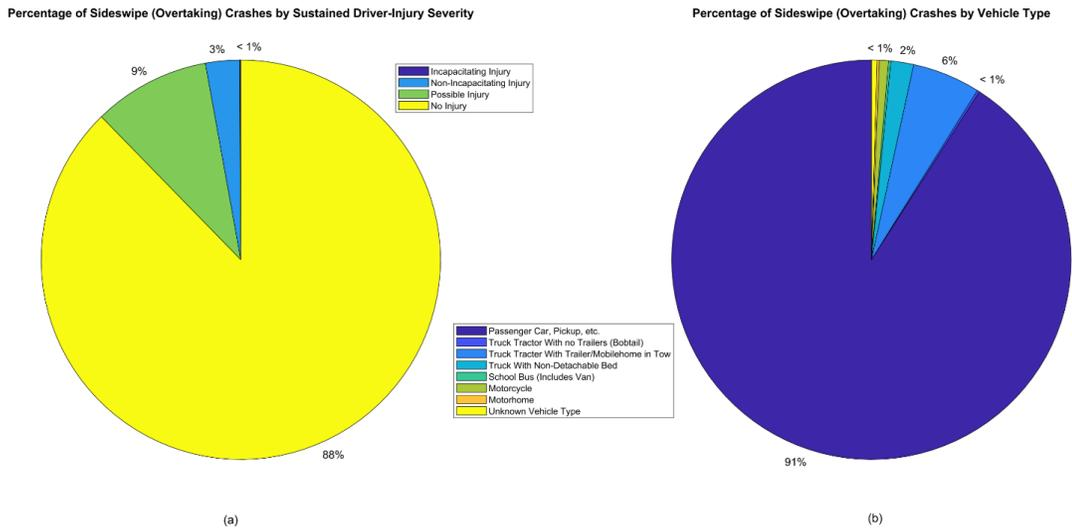
**Figure 3.21: Percentage of Sideswipe (Overtaking) Crashes at Hard Braking Hot Spots by (a) Injury Severity and (b) Vehicle Type**
