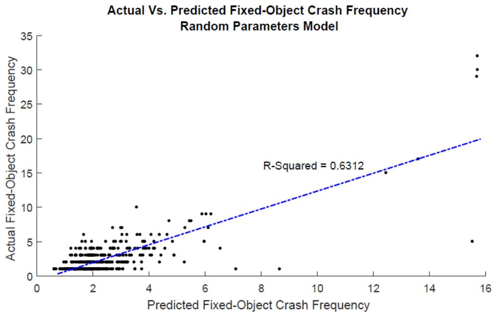
**Figure 6.5: Actual Versus Predicted Fixed-Object Crash Frequency for Random Parameters Poisson Model**
