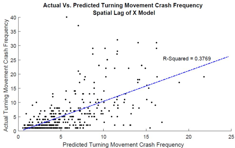
**Figure 6.4: Actual Versus Predicted Turning Movement Crash Frequency for SLX Negative Binomial Model**
