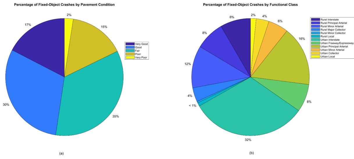
**Figure 3.18: Fixed-Object Crashes by (a) Pavement Condition and (b) Functional Class of Roadway**
