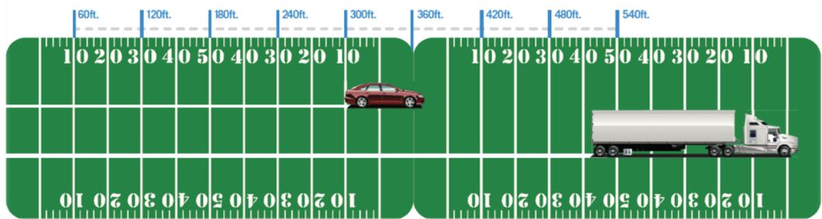
Figure 1.1: Comparison of Stopping Distances Between Passenger Vehicles and Heavy-Vehicles (Source: Utah Department of Transportation, 2018)
