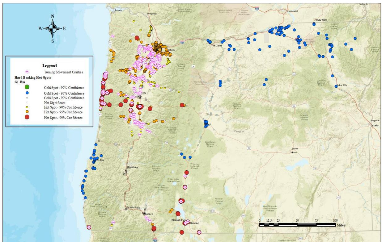
**Figure 3.10: Turning Movement Crashes at Heavy-Vehicle Hard Braking Hot Spots**
