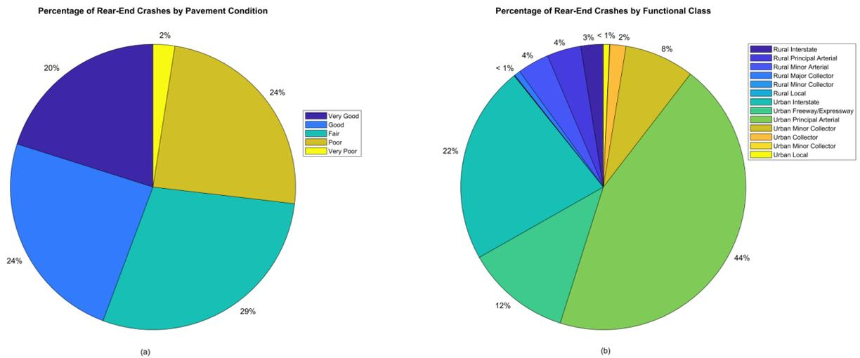
**Figure 3.8: Rear-End Crashes by (a) Pavement Condition and (b) Functional Class of Roadway**
