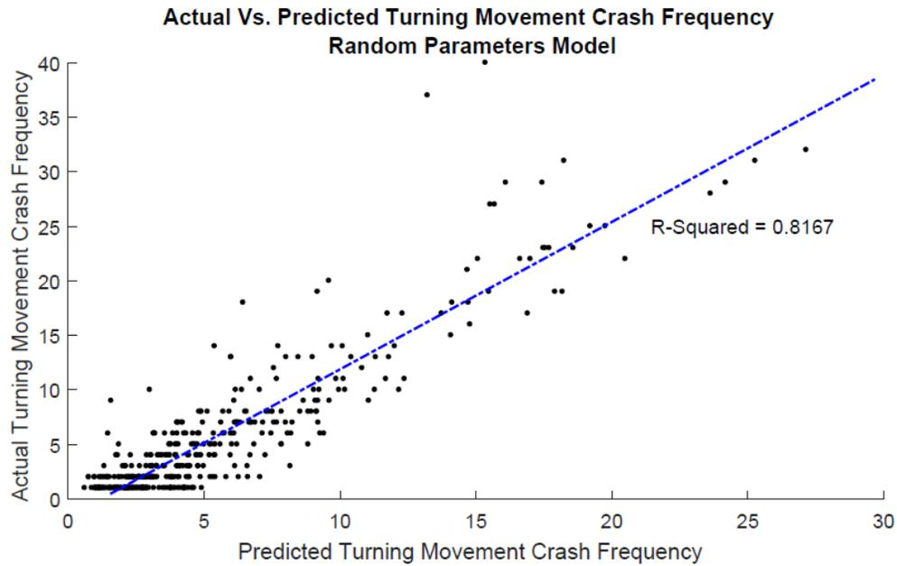
**Figure 6.3: Actual Versus Predicted Turning Movement Crash Frequency for Random Parameters Negative Binomial Model**
