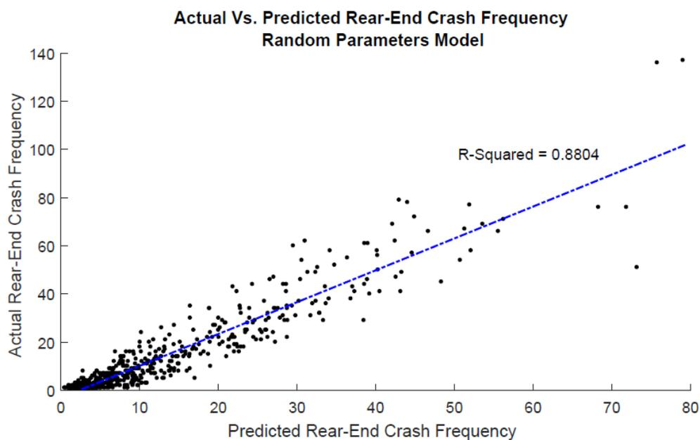
**Figure 6.1: Actual Versus Predicted Rear-End Crash Frequency for Random Parameters Negative Binomial Model**
