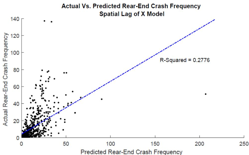
**Figure 6.2: Actual Versus Predicted Rear-End Crash Frequency for SLX Negative Binomial Model**
