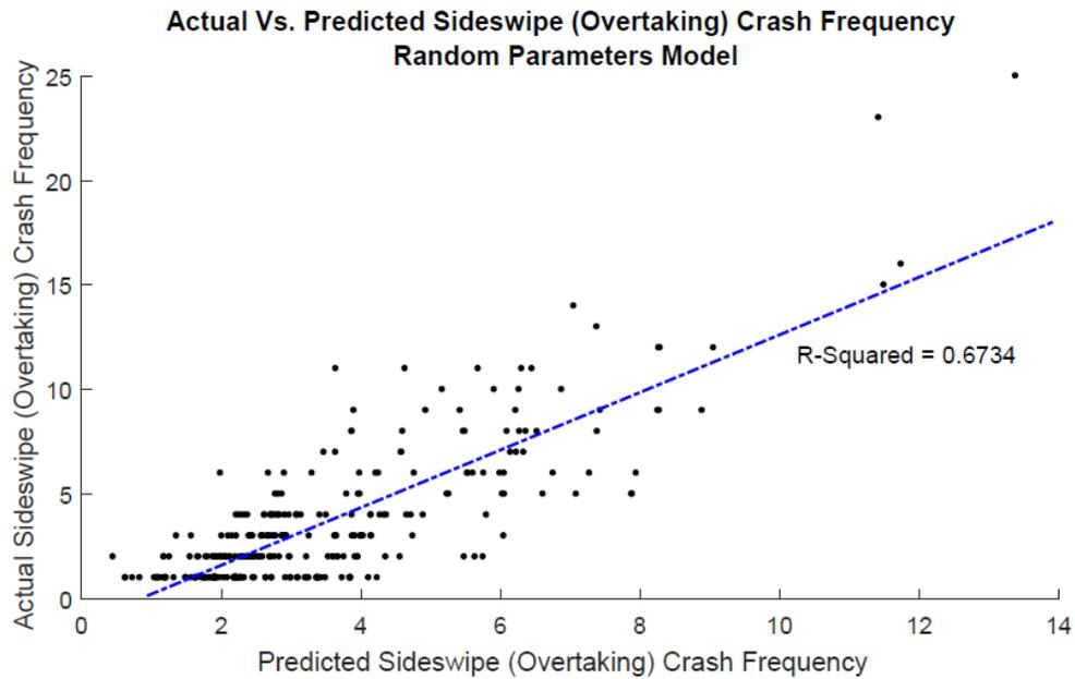
**Figure 6.7: Actual Versus Predicted Sideswipe (Overtaking) Crash Frequency for Random Parameters Negative Binomial Model**
