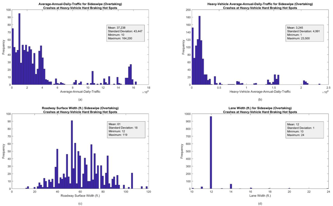
**Figure 3.22: (a) AADT, (b) T-AADT, (c) Roadway Surface Width, and (d) Lane Width for Sideswipe (Overtaking) Crashes**
