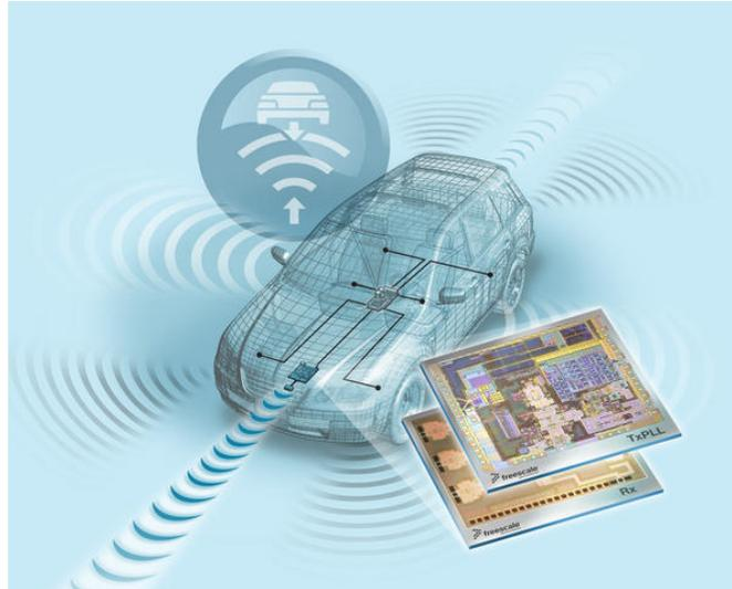
Figure 1.1: Commercialized 77 GHz silicon germanium (SiGe) BiCMOS transmitter for automotive radar (Freescale Semiconductor (now NXP) [1]).
