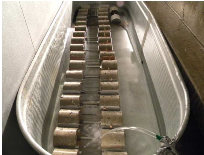
Fig. 8.4 – Bond specimens undergoing freeze-thaw effects and wet-dry conditions
