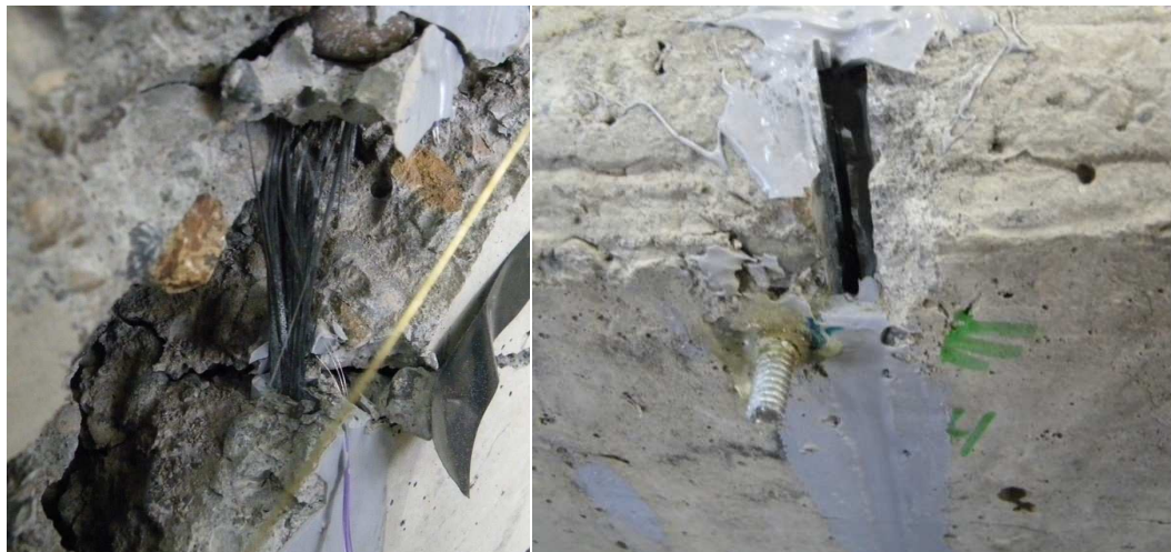
Fig. 6.4 – CFRP bending/rupture combination and slippage at the top of strip
