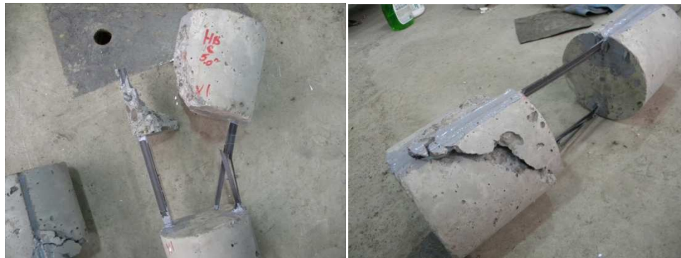
Fig. 8.2 – Failure of concrete around the NSM repair
