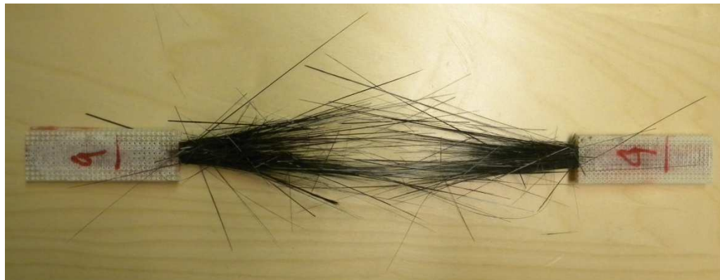
Fig. 4.9 – Example of desired CFRP coupon failure
