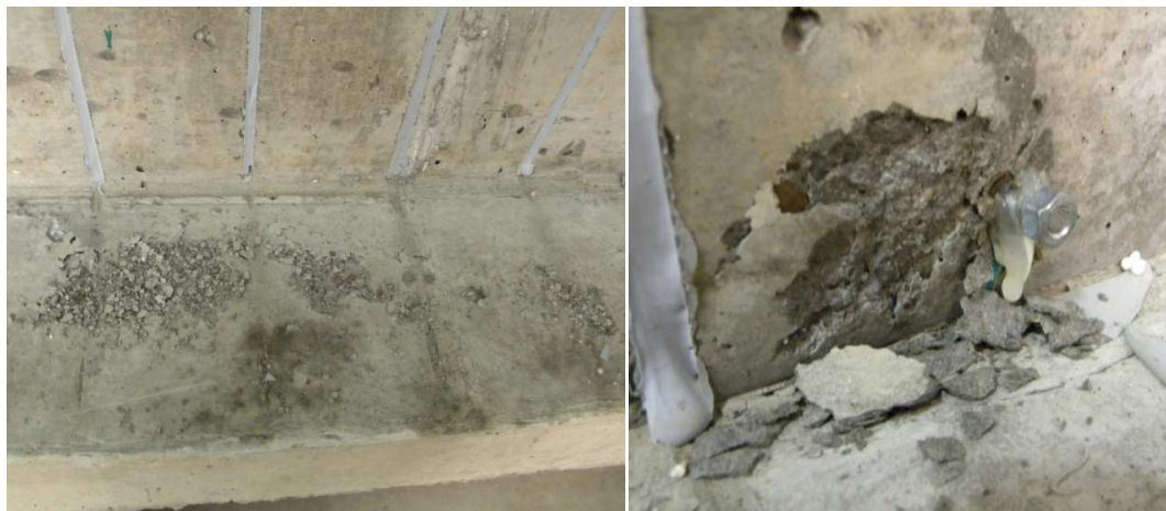
Fig. 6.6 – Specimen IT.7.22.6.FT effects from freeze-thaw exposure
