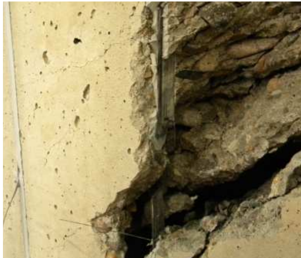
Fig. 6.7 – Rupture of CFRP strip without slippage
