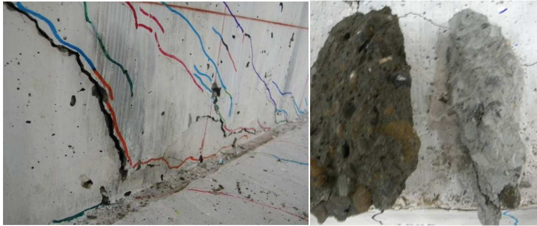
Fig. 6.5 – Specimen IT.7.18.6.M initial peeling and saturated concrete vs. dry concrete
