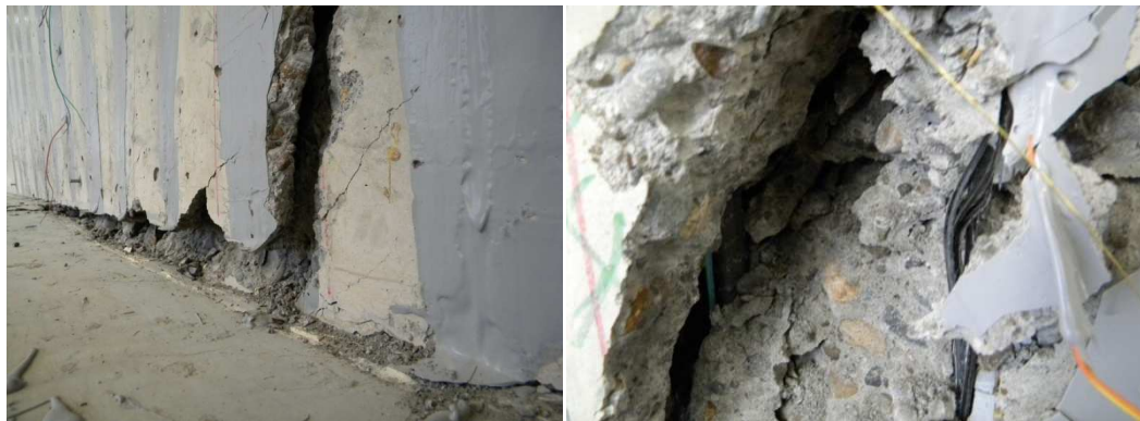
Fig. 6.2 – Specimen IT.7.18.6.S failing around the NSM retrofit and a bent CFRP strip
