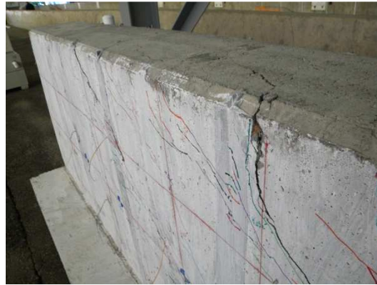
Fig. 6.1 - Specimen T.6.18.12.S was approaching a shear failure (specimen is inverted in photograph prior to loading on a truck for disposal)
