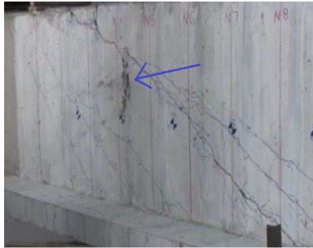
Fig. 6.3 – Concrete failing around CFRP strip just prior to shear failure
