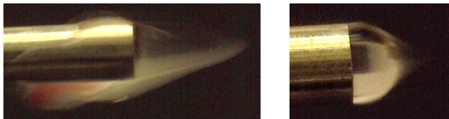
Figure 4.3: Electrospray using 40Hz sine wave pulse with 4kVpp and 4kVdc at a 3 cm distance from needle to substrate. (Left) Electrospray at a silicon wafer chip substrate. (Right) 500µm diameter platinum electrode.
