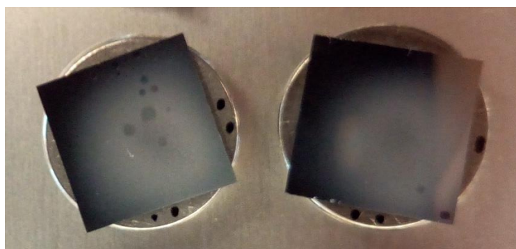
Figure 2.1: Electrospray deposition onto 1cmx1cm silicon wafer coupons. Here mounted on pin stub holders prior to SEM imaging.
