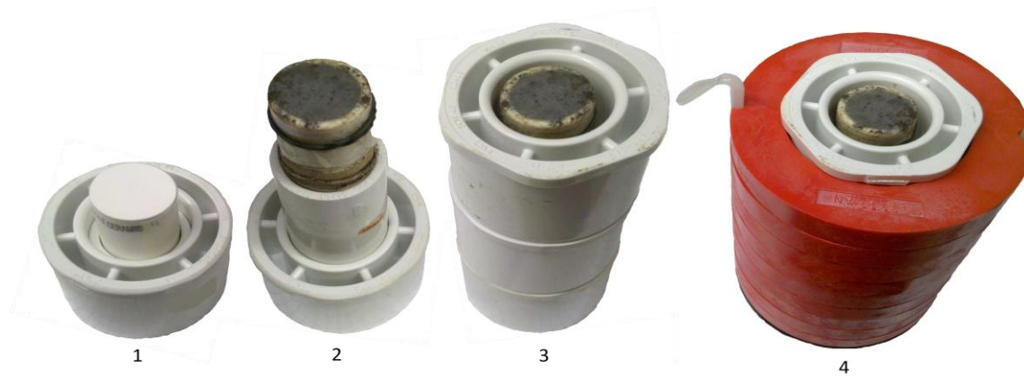
Figure 3: Stepwise assembly for centrifugation. Step 1.) the ceramic rod is placed in a PVC holder. Step 2.) the soil core is placed atop the ceramic and held in place with a PVC coupling. Step 3.) The entire setup is held in place with additional PVC fittings. Step 4.) The assembly is placed within the Multi-Disc rotor bucket holder adapter.
