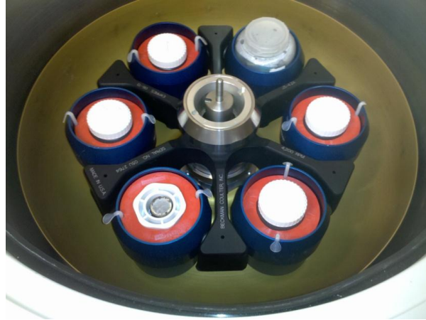
Figure 2: Avanti J-HC centrifuge with JS-4.2A rotor. The sampling device is loaded on bottom left bucket with the remaining buckets containing counterweights.
