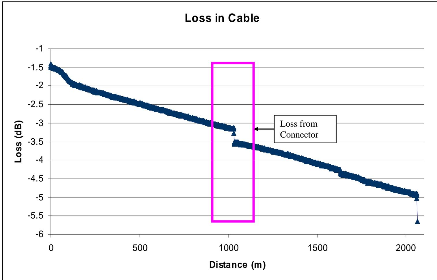
Figure 5.2 High loss cable (acceptable loss is 1dB/ km) and an approximate 0.5 dB loss encountered at a barrel connector at 1030 and 0.75 dB loss at the barrel connector at 2060 meters.
