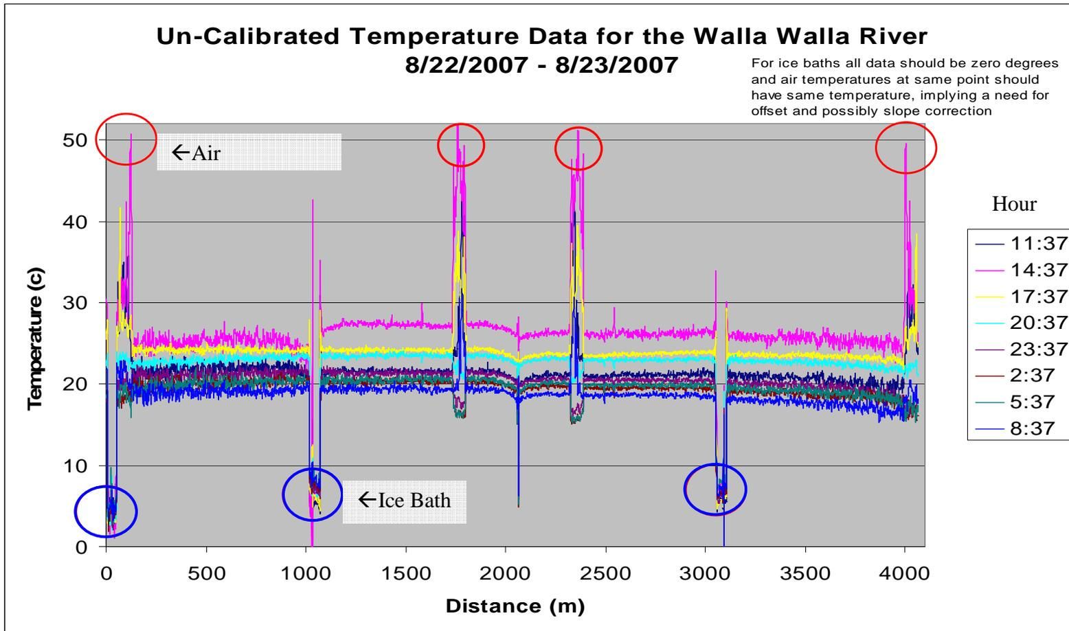
Figure 4.1 The un-calibrated graph shows eight hours of temperature profile for the reach. The duplex cable used shows a mirrored image after 2060 meters. Blue circles indicate ice baths and red circles locations of known air exposed sections of cable.
