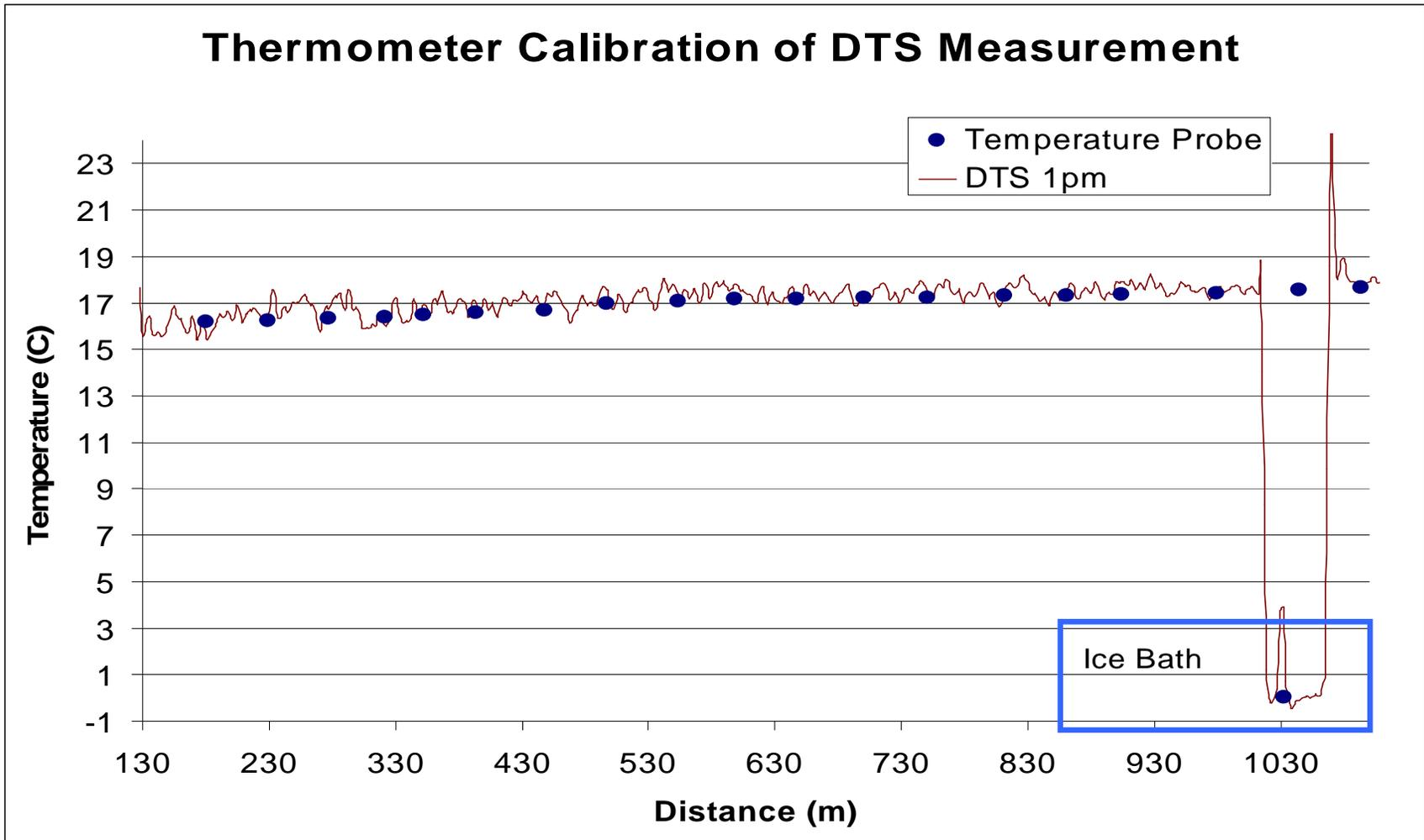
Figure 3.4 High precision temperature probe measurements compared to DTS measurements for 1000m of the study reach at 1pm.
