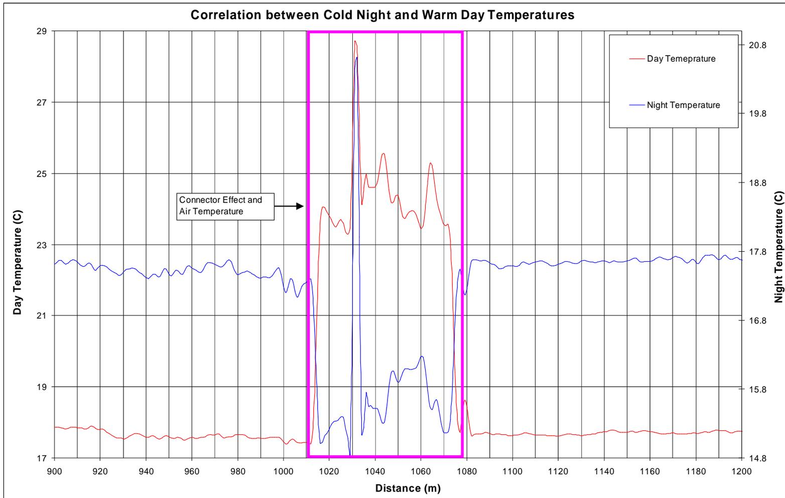
Figure 5.3 Air temperature and barrel connector site from the temperature profile, the barrel connector is the large spike during both the night and day at 1030 m.
