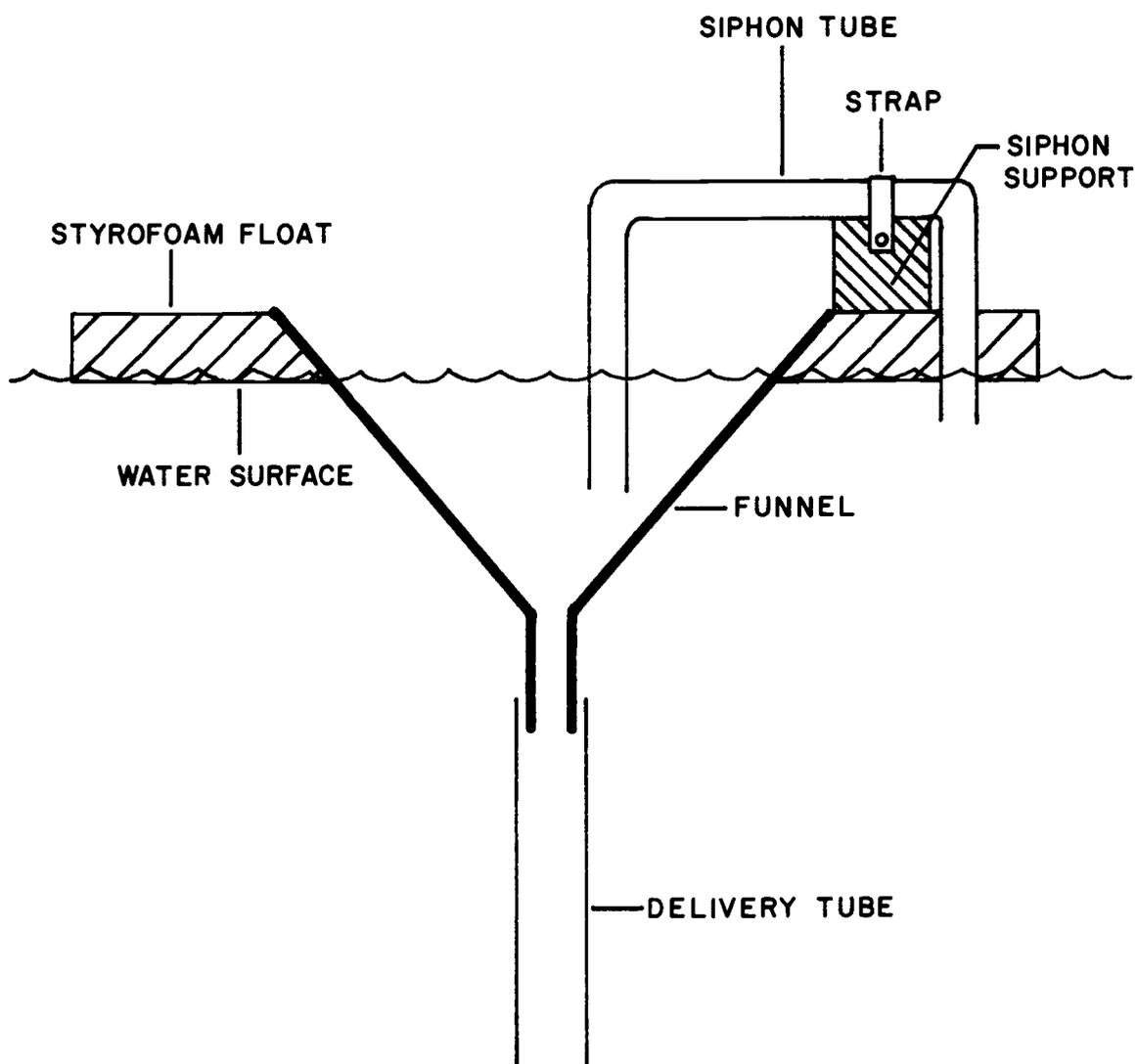
Figure 2. Diagram of the constant flow device for delivery of turbid water to exposure chambers (after Freeman, 1971).
