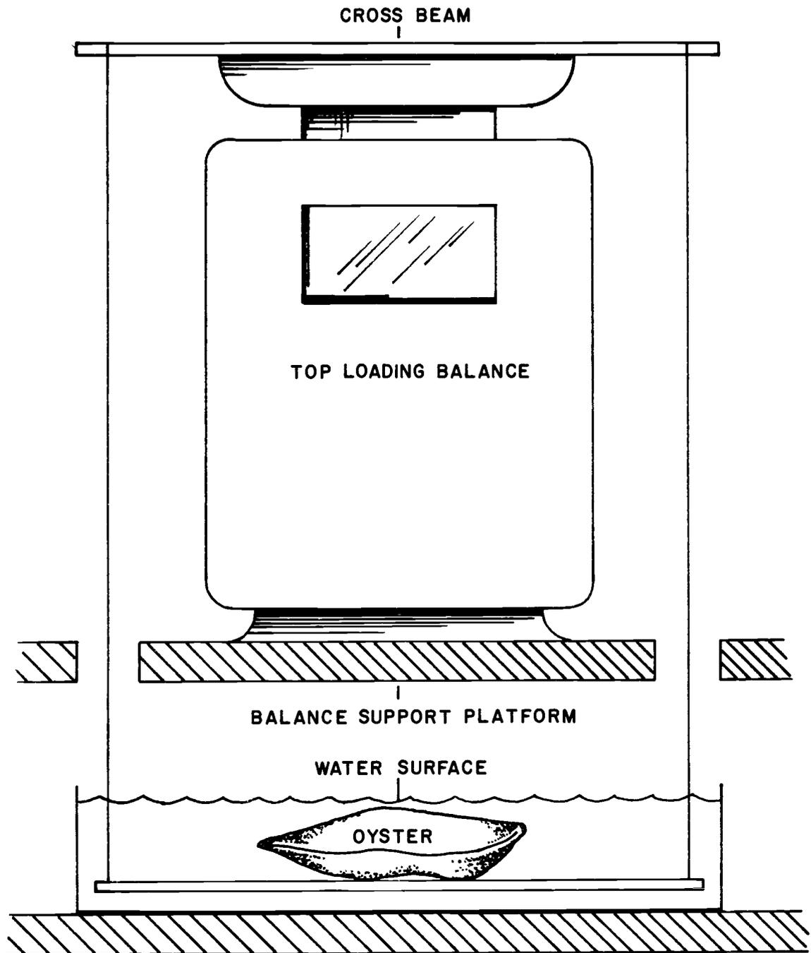
Figure 5. Modified top-loading balance used for weighing oysters under water.
