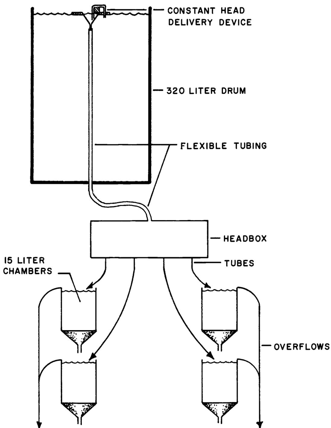
Figure 1. Design of the sediment exposure units used in the growth studies.
