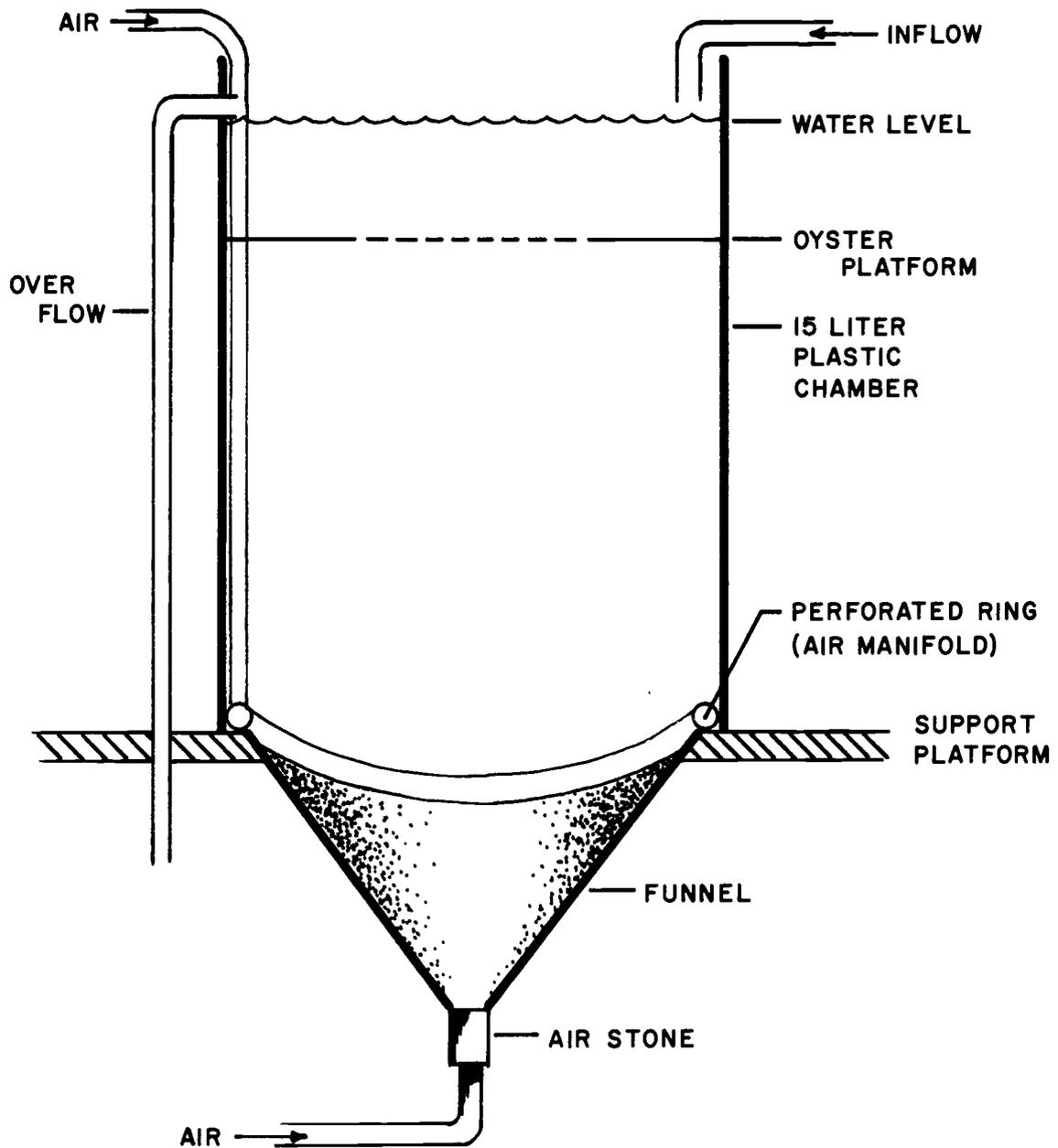
Figure 3. Diagram of an exposure chamber showing details of the aeration system for keeping sediments in suspension.
