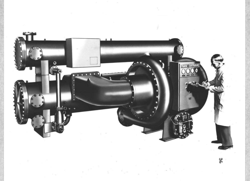
Vanes are located at the inlets of both the first stage and second stage impellers to modulate the refrigerant gas; this regulates the load carried by the machine. These vanes are connected, through a ring and gear mechanism, to an automatic air diaphragm operator which is controlled, in turn, by external air pressure. The variation of the air pressure which is caused by changing load, will be described in chapter five in the section on controls. (43, p.8)
