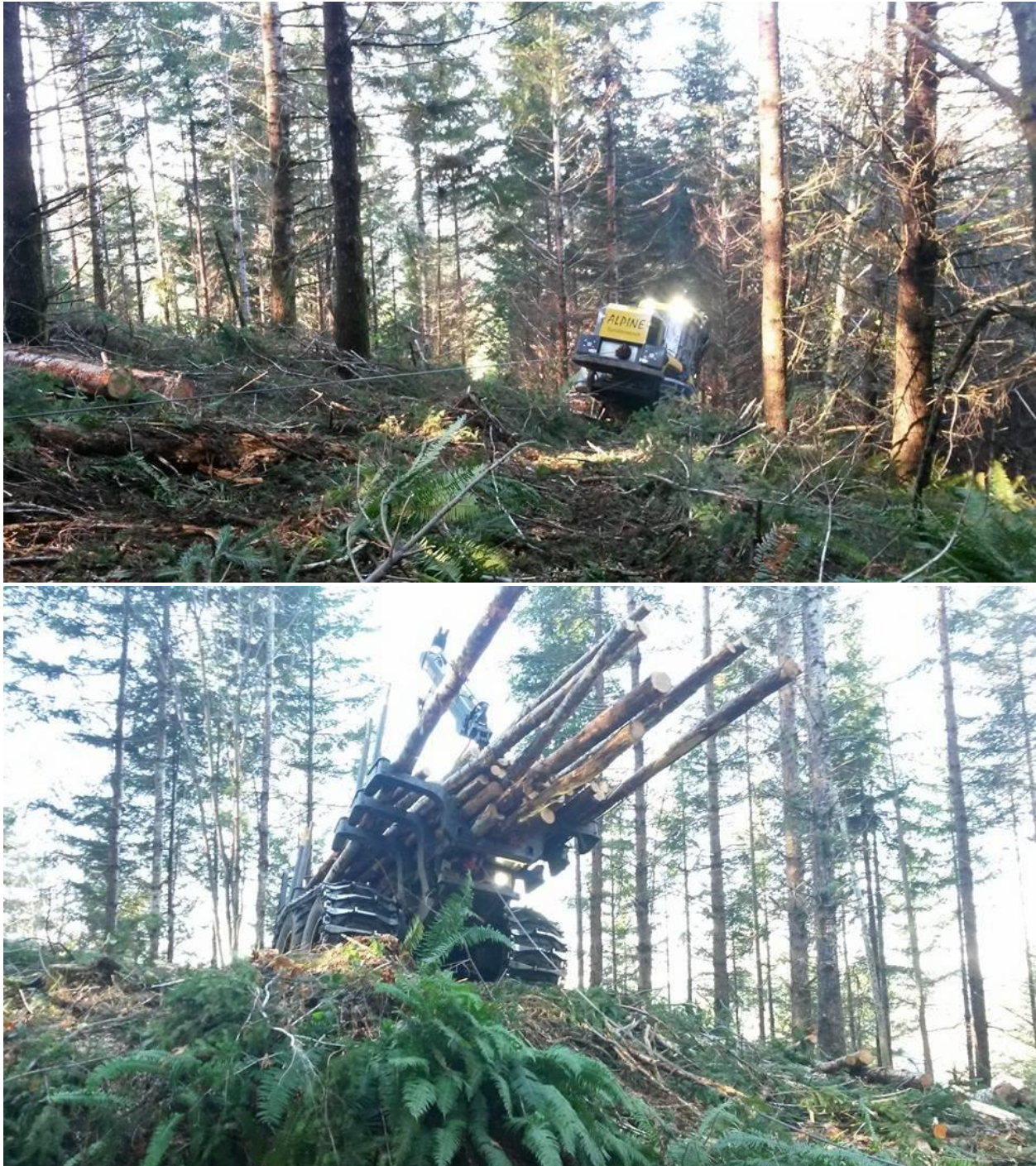
Figure 2.2: Ponsse Bear harvester (above) and Elephant King forwarder (below) on tethered thinning operations in the Oregon Coast Range
