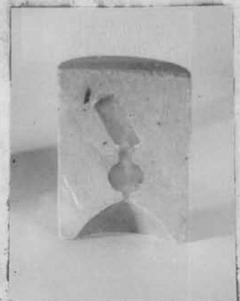
(Cut away view) Mold ready for burn-out
