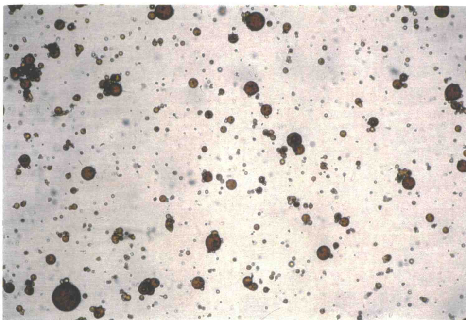
Figure 3.1: Sudan III-stained spray microcapsules (SMs) composed of 60% w/w tripalmitin/40% w/w fish oil. SMs recovered from control beakers after 6 hours suspension in seawater at 12°C. SMs were spherical and red in color. SMs did not accept blue counter-stain (Nile-blue sulfate). Magnification, 160X objective. Scale _____ = 50 \mu\text{m} .
