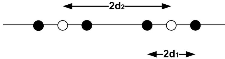
Figure 4.4: Superimposed BPSK constellation.  $2d_1$  is the distance between  $s_1$  and  $2d_2$  is the distance between  $s_2$ .
