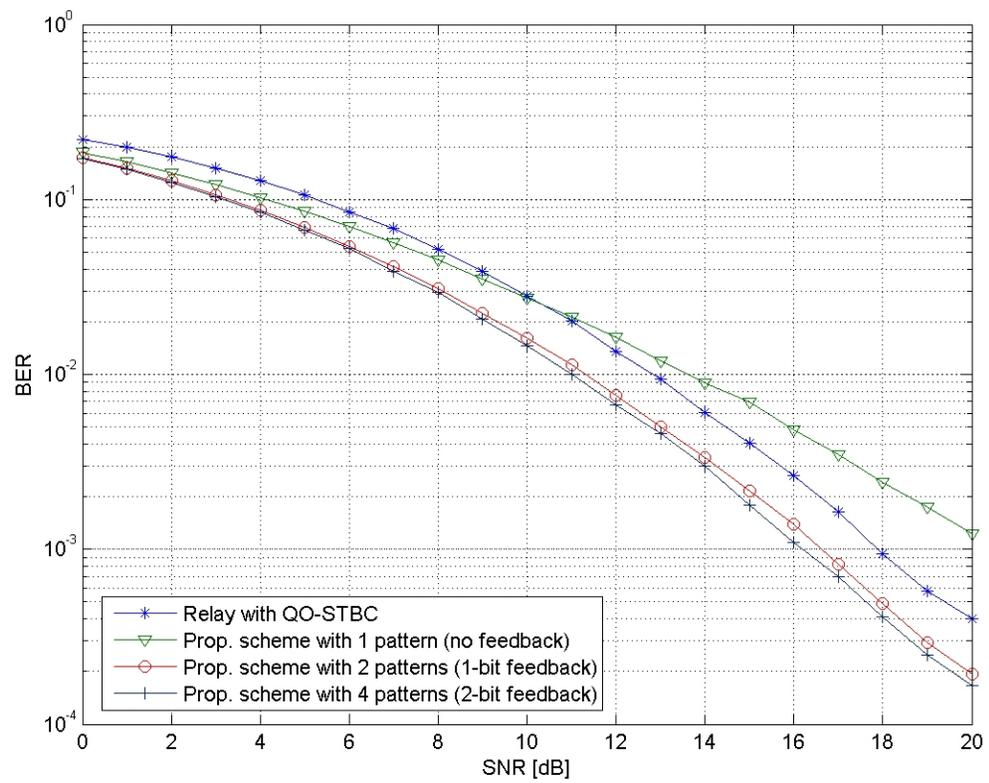
Figure 2.4: BER performance of the proposed system with an MMSE receiver.
