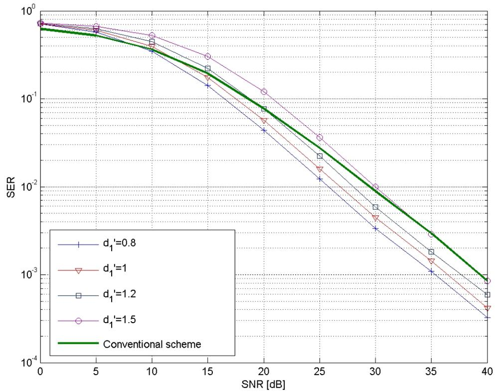
Figure 5.10: The SER performance of mobile 1 (enhancement bits are assigned to mobile 1 and common bits are assigned to mobile 2): Asymmetric model.
