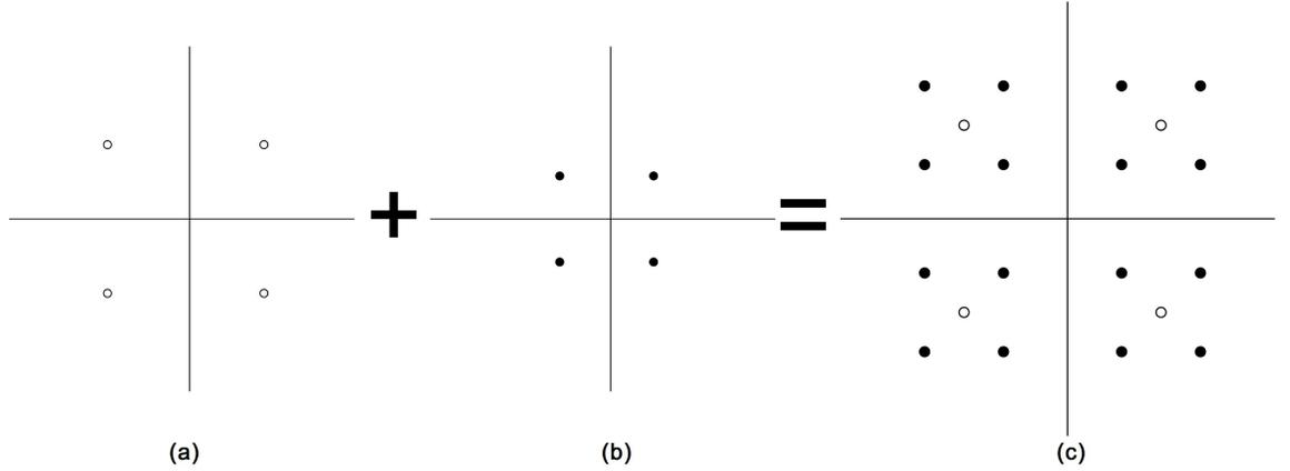
Figure 3.3: Superposition encoding. The power of  $x_1$  is  $\sqrt{1-\alpha}$  and the power of  $x_2$  is  $\sqrt{\alpha}$ .
