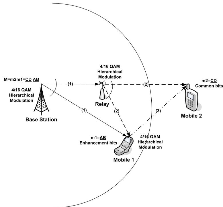
Figure 5.9: Hierarchical modulation based cooperative multiuser communication: Asymmetric model.
