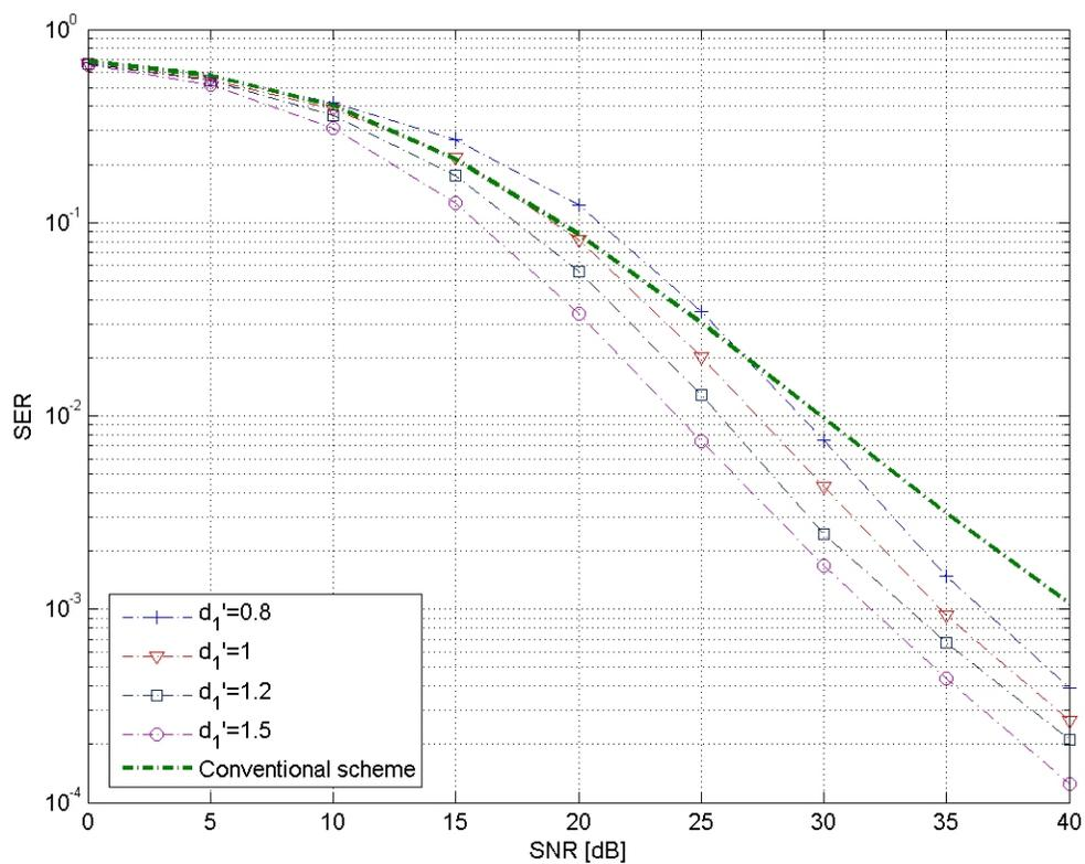
Figure 5.11: The SER performance of mobile 2 (enhancement bits are assigned to mobile 1 and common bits are assigned to mobile 2): Asymmetric model.
