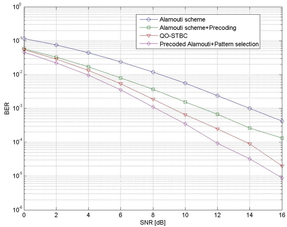
Figure 2.1: Bit error performance of different four-transmit antenna systems
