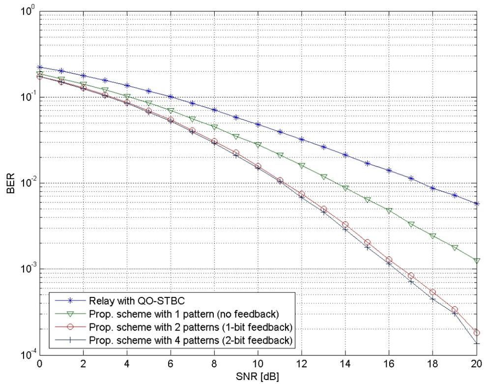
Figure 2.5: BER performance of the proposed system with a ZF receiver.
