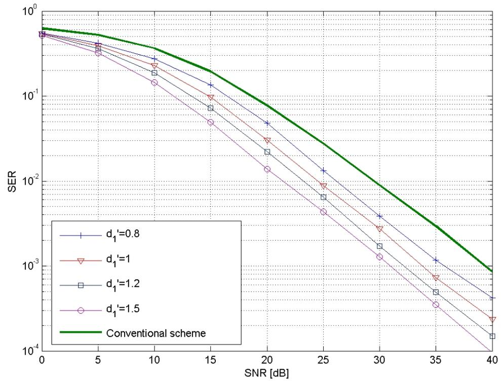
Figure 5.12: The SER performance of mobile 1 (common bits are assigned to mobile 1 and enhancement bits are assigned to mobile 2): Asymmetric model.
