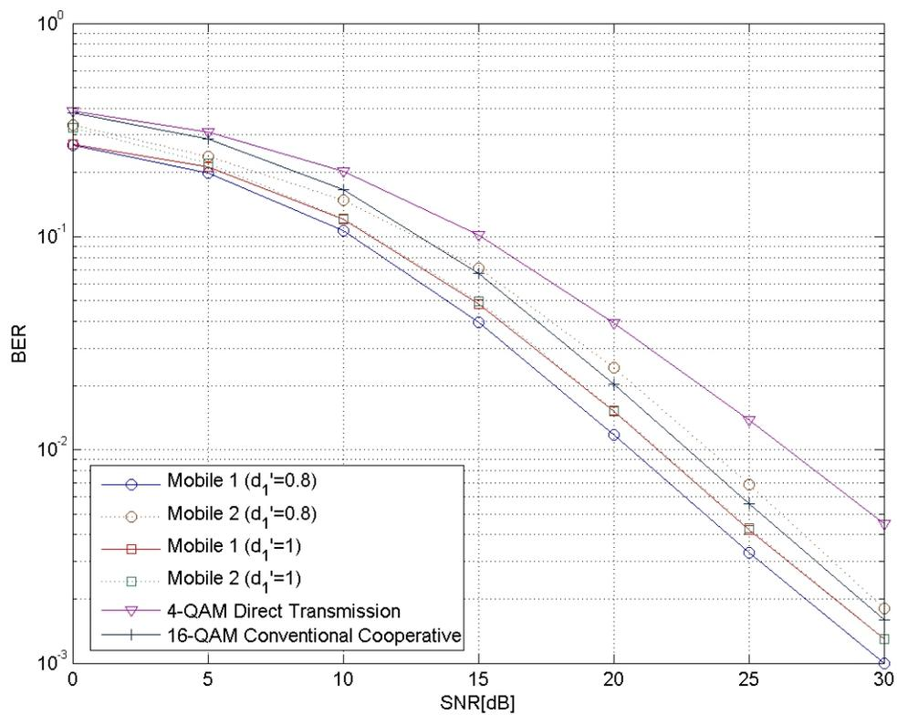
Figure 5.7: The BER performances of mobile 1 and mobile 2
