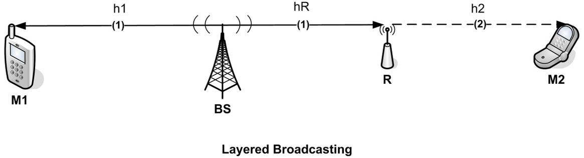
Figure 3.4: Proposed Downlink transmission system.
