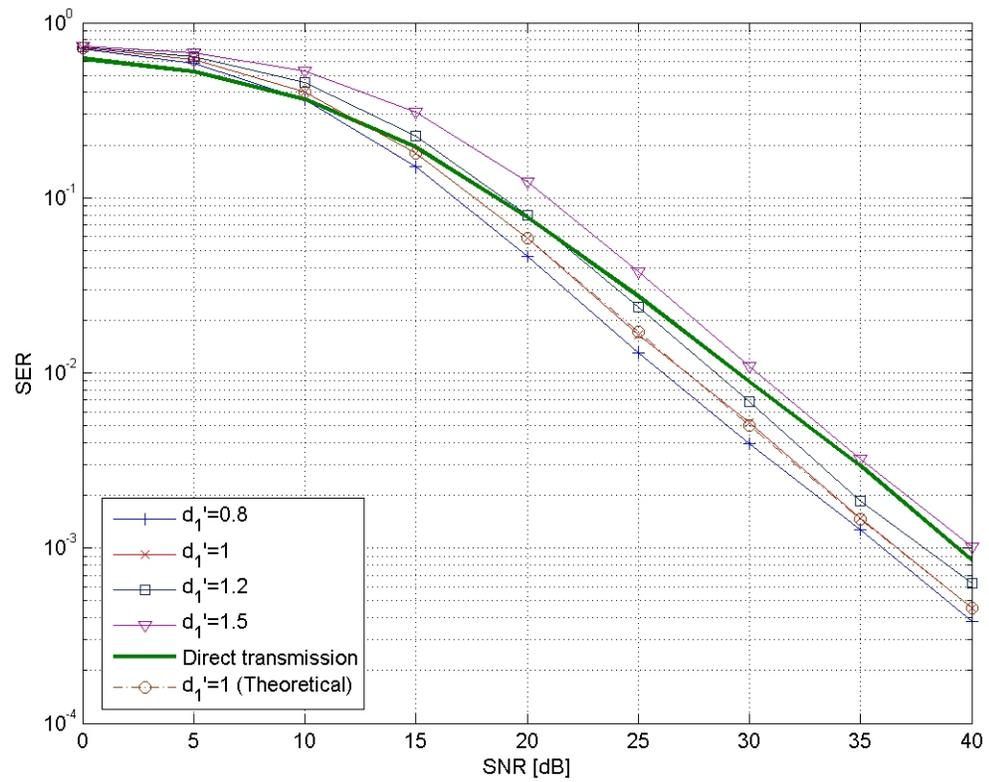
Figure 5.5: The SER performance of mobile 1 (enhancement bits are assigned to mobile 1 and common bits are assigned to mobile 2): Symmetric model.
