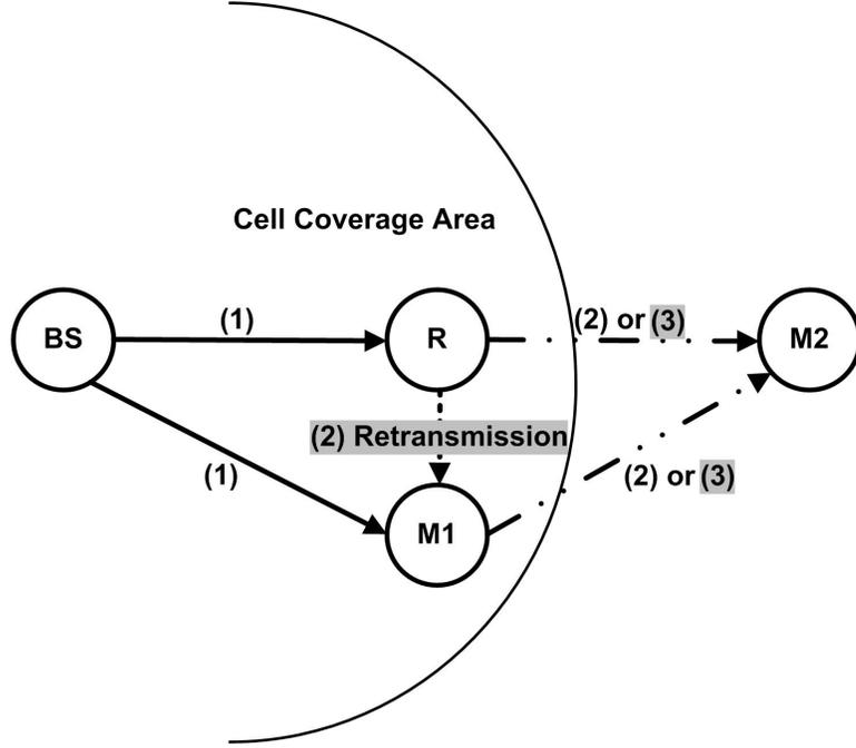
Figure 4.3: Proposed Scheme: Superposition coding plus relay transmission (2-transmission phases without retransmission or 3-transmission phases with retransmission)
