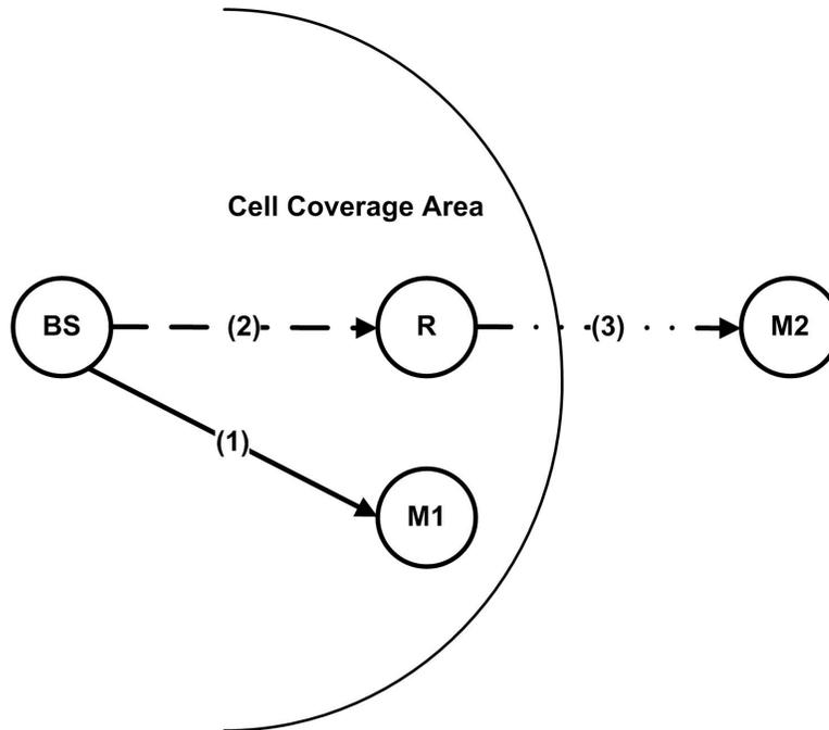
Figure 4.1: Conventional Downlink Transmission System: Direct Transmission + Relay Transmission (3-transmission phase)
