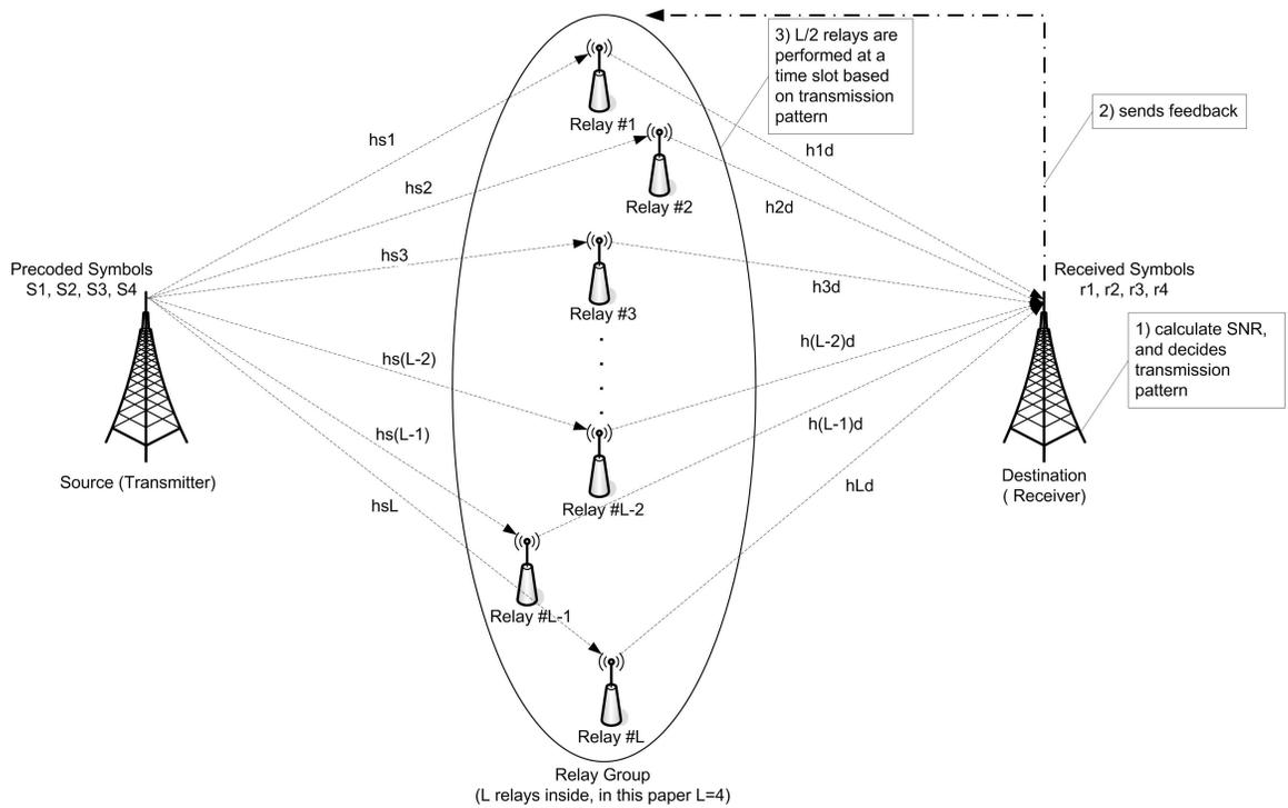
Figure 2.2: Single-hop relay communication system model.
