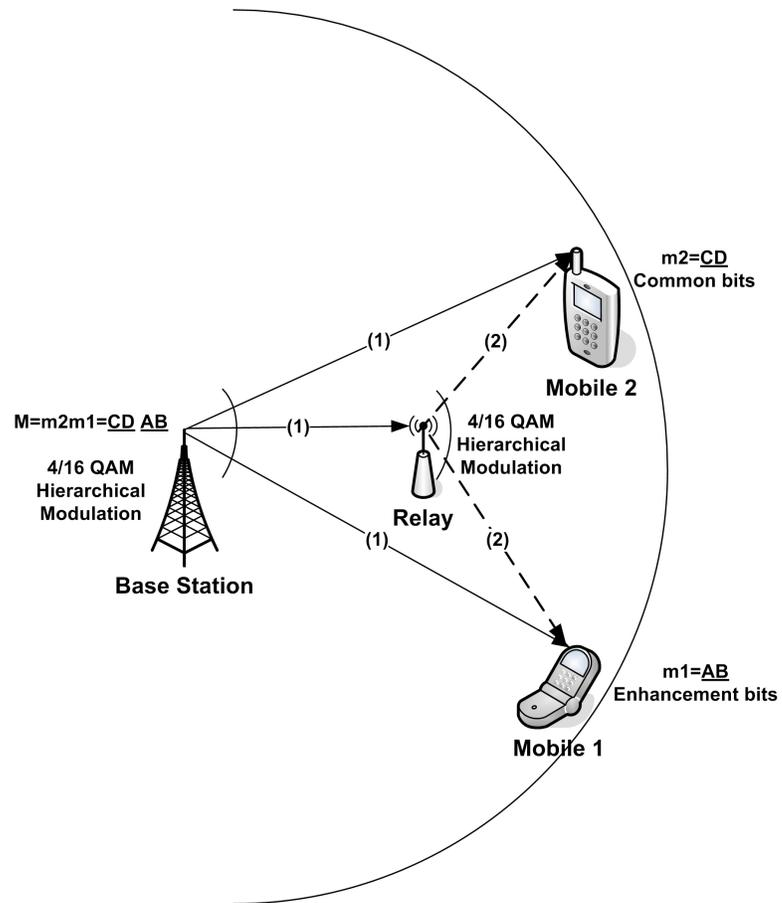
Figure 5.3: Hierarchical modulation based cooperative multiuser communication: Symmetric model.
