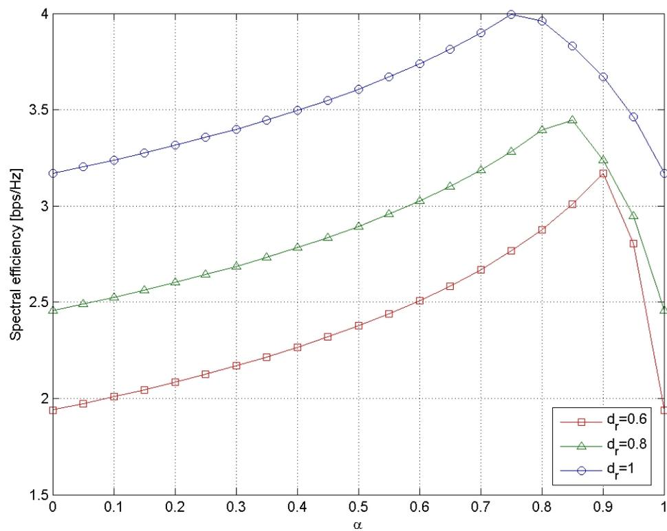
Figure 3.6: The spectral efficiency according to the value of  $\alpha$  ( $\gamma_0 = 20dB$ ).
