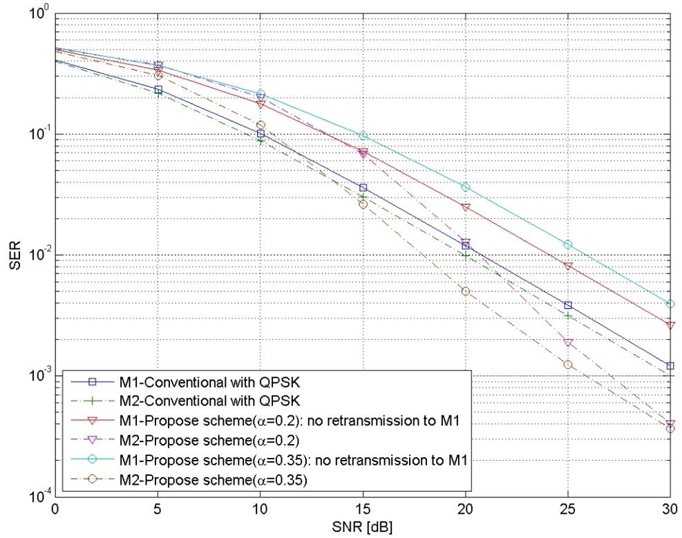
Figure 4.5: The SER performance of the proposed system with no retransmission from R to M1:  $s_1$  is assigned as basic message and  $s_2$  is assigned as superposed message.
