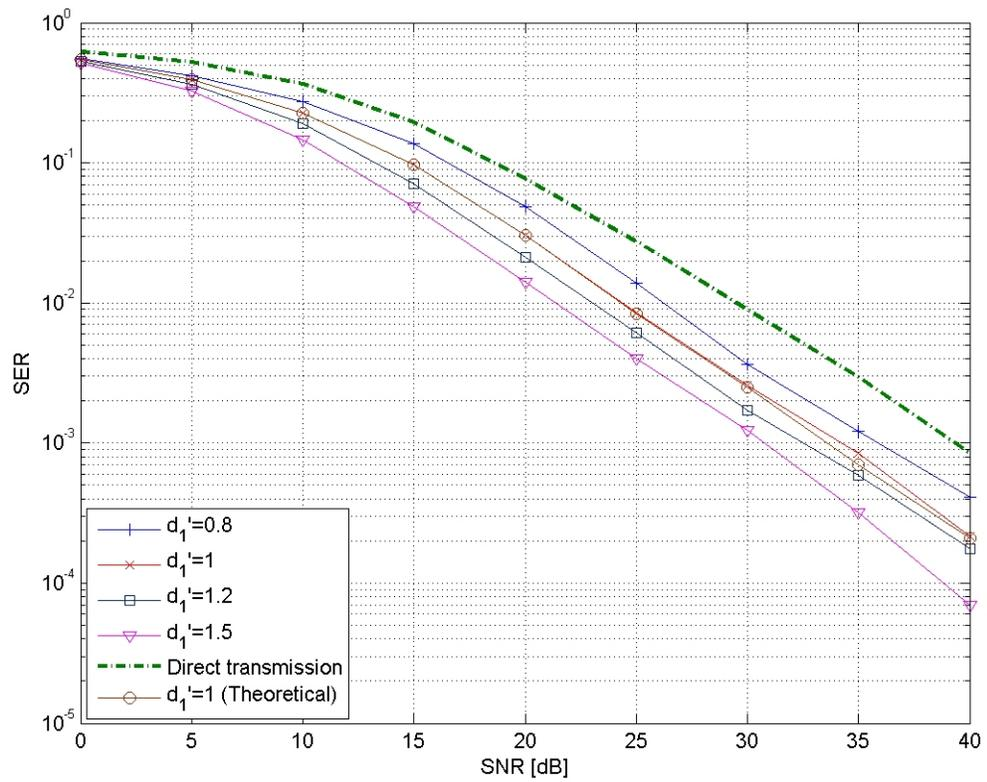
Figure 5.6: The SER performance of mobile 2 (enhancement bits are assigned to mobile 1 and common bits are assigned to mobile 2): Symmetric model.
