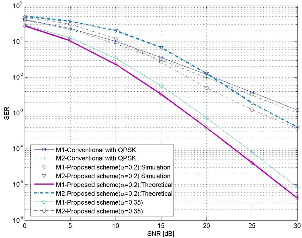
Figure 4.6: The SER performance of the proposed system:  $s_1$  is assigned as basic message and  $s_2$  is assigned as superposed message.
