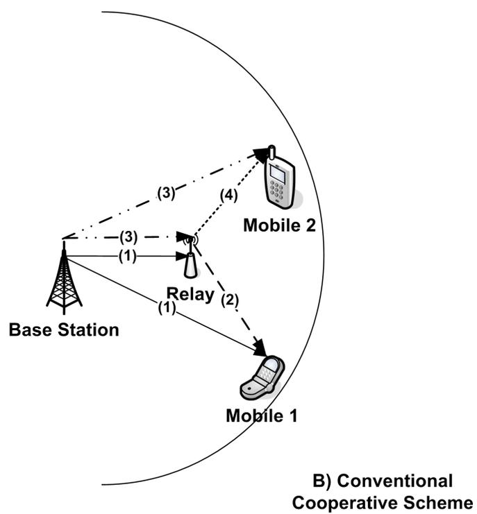
Figure 5.1: Conventional communications schemes: All mobiles are in cell coverage area.
