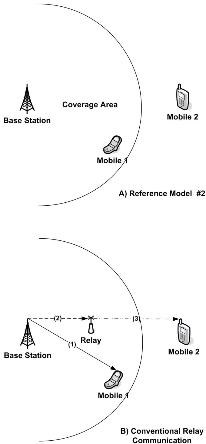
Figure 5.8: Conventional communications schemes: one mobile is out of cell coverage area.
