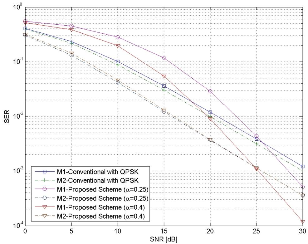
Figure 4.7: The SER performance of the proposed system:  $s_2$  is assigned as basic message and  $s_1$  is assigned as superposed message.
