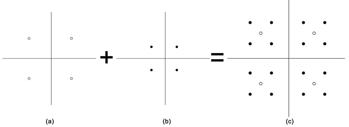
Figure 4.2: Constellation for superimposed QPSK. The circles and black symbols denote the constellations of  $s_1$  and  $s_2$  respectively. The power of  $s_1$  is  $\sqrt{E(1-\alpha^2)}$  and the power of  $s_2$  is  $\sqrt{E\alpha^2}$ .
