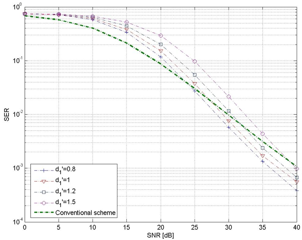
Figure 5.13: The SER performance of mobile 2 (common bits are assigned to mobile 1 and enhancement bits are assigned to mobile 2): Asymmetric model.
