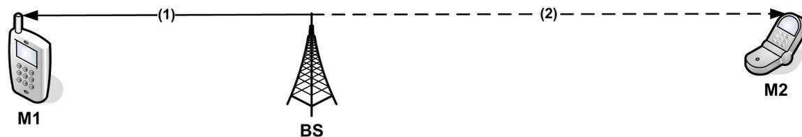
(a) Standard two-user forward link channel model
