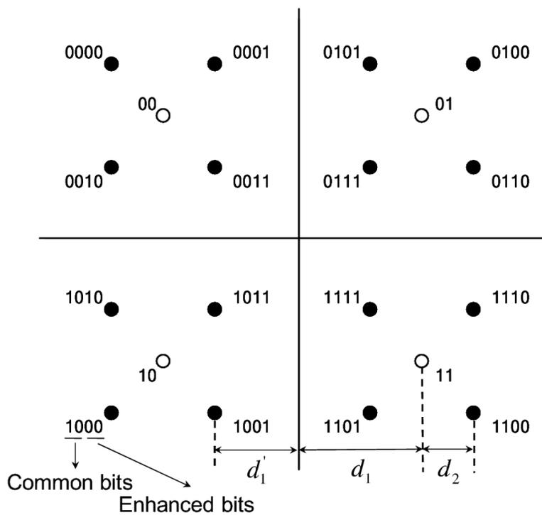
Figure 5.2: Constellation of 4/16-QAM hierarchical modulation.
