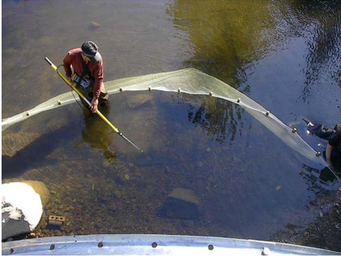
Figure 4. The seine is the limit of the Crane cold refuge area. The brick at lower left is attached to a temperature logger. The edge of the culvert seen in the bottom of the photo hangs over the confluence of Crane Creek and West Fork Smith River.
