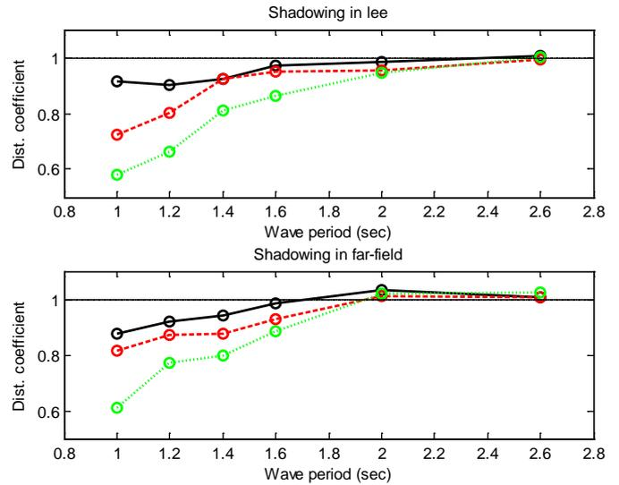
Fig. 7 Relative wave height vs wave period at (top) the lee gage array ( $\pm 1.5$  m from basin centreline) and (bottom) the far-field gage array ( $\pm 2$  m from basin centreline) as a function of WEC-array configuration, 1-device (black/solid), 3-device (red/dashed), and 5-device (green/dotted).
