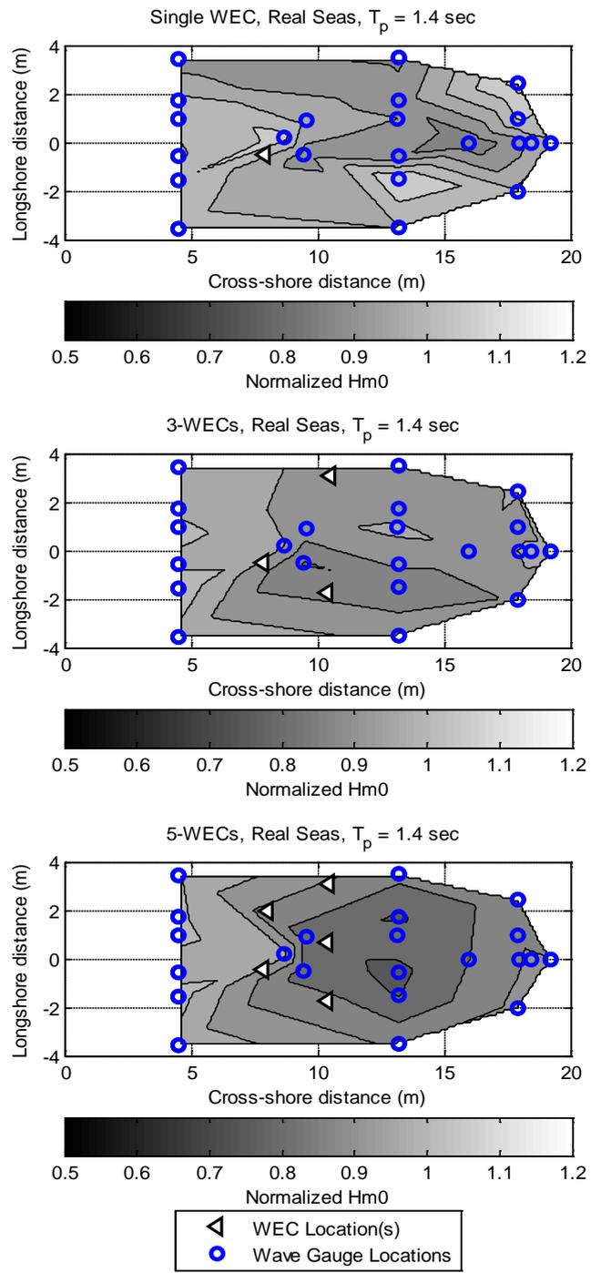
Fig. 5 Spectrally-determined relative wave heights,  $H_{m0}$ , measured across the domain for 1/3/5-WEC array (top), (middle), and (bottom), respectively. Real seas,  $T_p=1.4$  sec, peak incidence angle is shore normal, directional spreading factor  $s=4$ . Contour interval is 0.05 and contours were interpolated between measurements.
