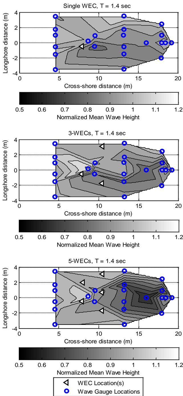
Fig. 4 Relative wave heights measured across the domain for 1/3/5-WEC array (top), (middle), and (bottom), respectively. Regular waves were normally incident,  $T=1.4$  sec. Contour interval is 0.05 and contours were interpolated between measurements.
