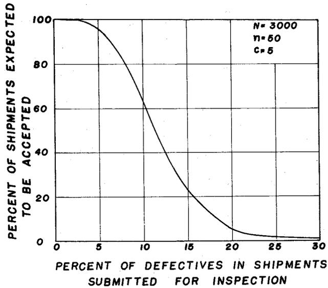
Figure 1 - Operating characteristic curve for an acceptance sampling plan with  $N = 3000$ ,  $n = 50$ , and  $c = 5$ .
