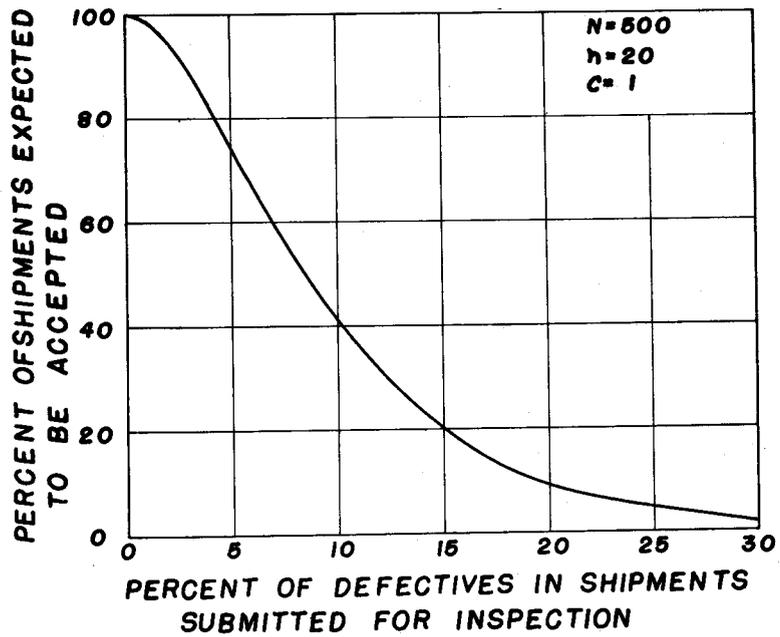
Figure 5 - Operating characteristic curve for an acceptance sampling plan with  $N = 500$ ,  $n = 20$ , and  $c = 1$ . For use with the simulated cars of  $2 \times 10$ 's.
