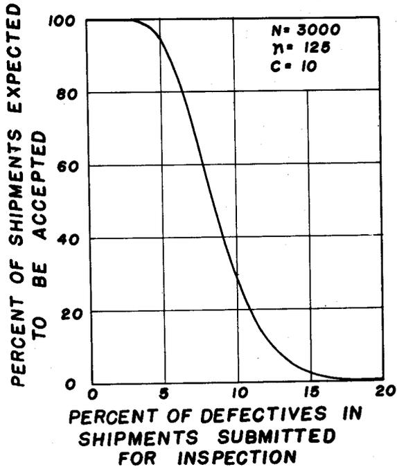
Figure 4 - Operating characteristic curve for an acceptance sampling plan with  $N = 3000$ ,  $n = 125$ , and  $c = 10$ .
