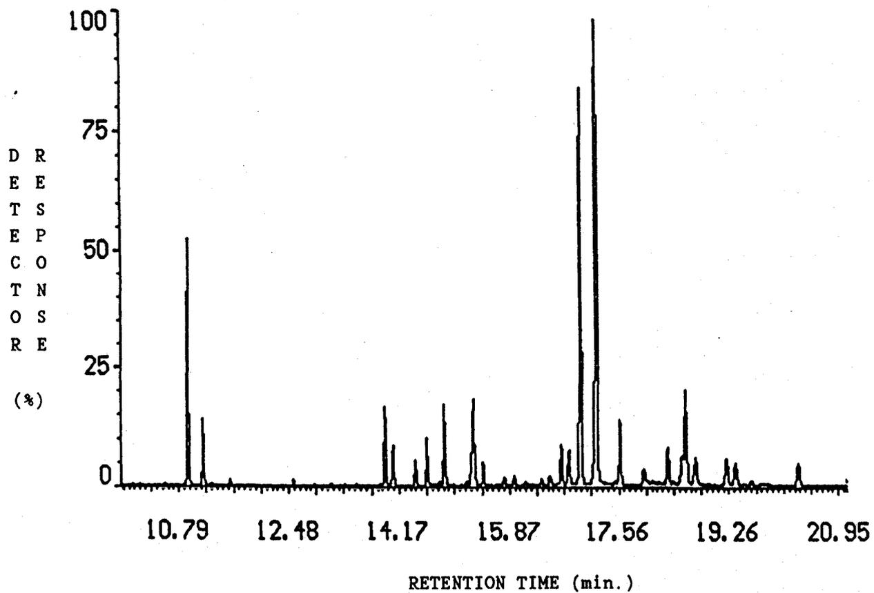
Figure 15(a). GC of ether extracts of lumber stained sapwood
