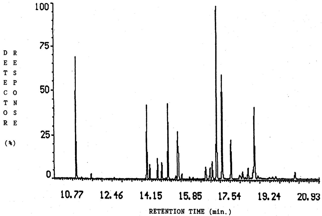
Figure 15(b). GC of ether extracts of timber nonstained sapwood
