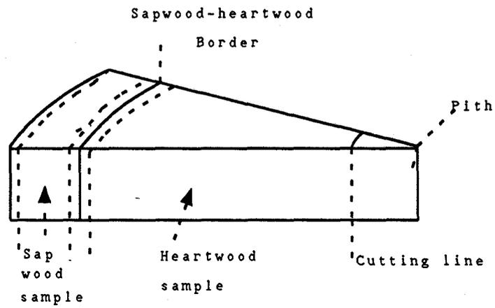
Each sample of sapwood and heartwood was cut into small pieces and ground in a Thomas-Wiley lab mill to pass through the 40 mesh screen of the mill.
