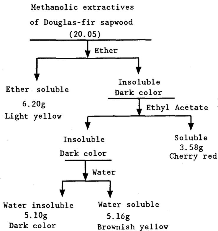
Figure 6. Partition of the heartwood extractives with solvents.
