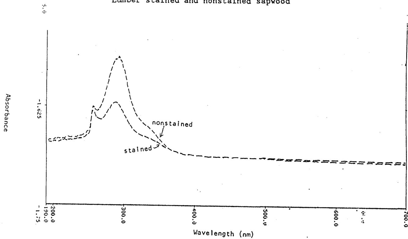
Figure 11. UV-Visible absorption of Douglas-fir wood extractives
