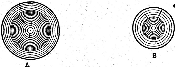
Figure 1. Post A has a greater percentage of heartwood than B, therefore is more desirable as a fence post.
