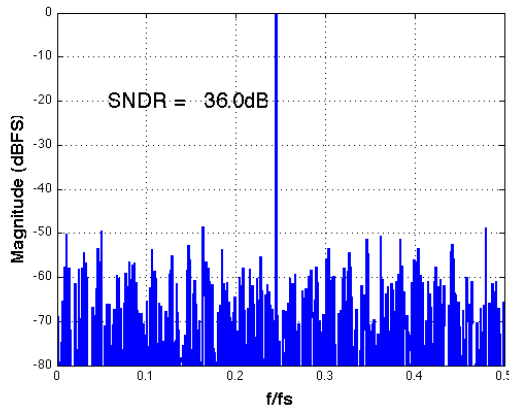
Fig. 2-4. The 8192-length FFT of a 6-bit pipeline SAR ADC with 200 fF sampling capacitor and 2 fF parasitic capacitance at the input of a comparator.
