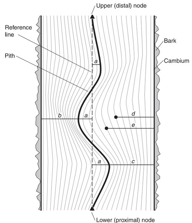
Fig. 1, *a*) to either side of the line was then recorded. For the largest pith deviation to each side of the reference line we measured the distance from the cambium to the outer edge of the pith (Fig. 1, *b* and *c*). The pith was noted as offset if it had a distinct J shape, most likely as a result of damage to the bud or leader, but it was still counted as a pith deviation.
