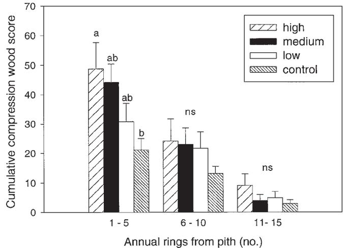
more severe CW near the pith, the impact lessened substantially toward the bark, suggesting that the higher quality outer wood remains unaffected. This pattern may explain why Middleton et al. (1989) found no connection between sinuosity and drying degrade.
