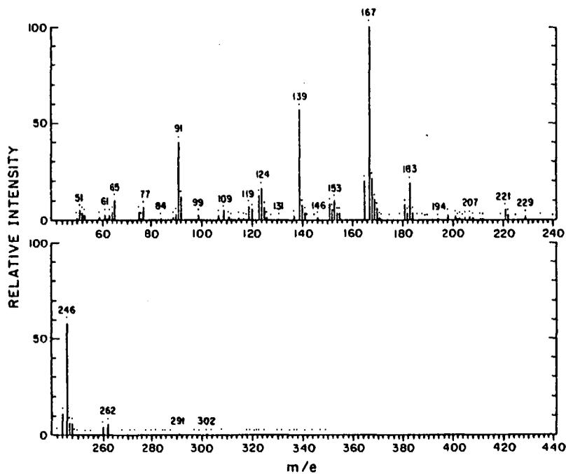
Figure 7. Mass Spectra of Mesurol sulfide mesylate detected in Pinot Noir wine produced from field treated grapes.
