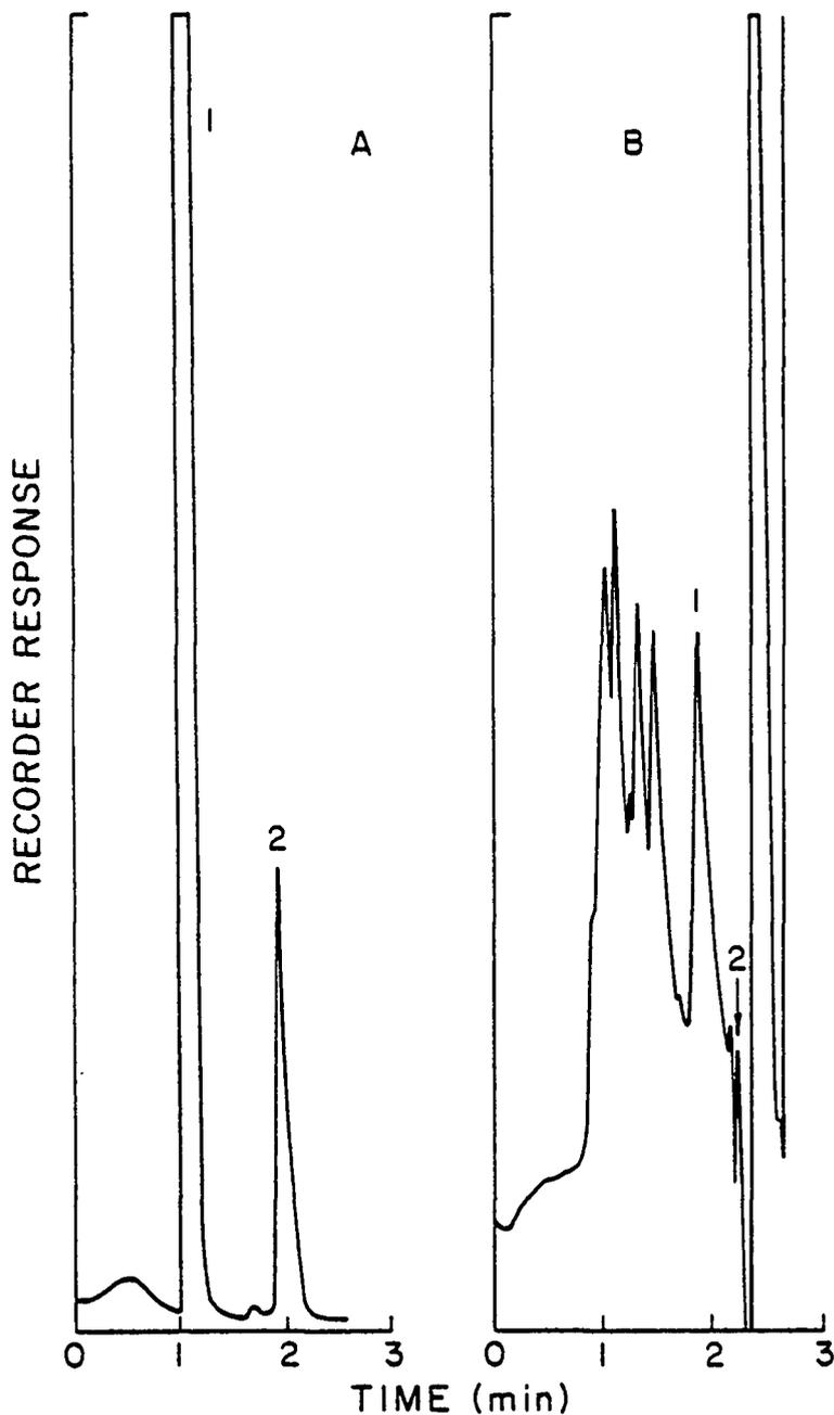
Figure 5. Representative HPLC chromatograms. Attenuation - 4X. Flow rate - 2 ml/min. (A) Mesurol sulfide phenol (peak 2) in benzene (peak 1). (B) Mesurol treated Pinot Noir wine. Peak 1 was collected. Flow rate was increased to 3 ml/min after peak 2 had eluted.
