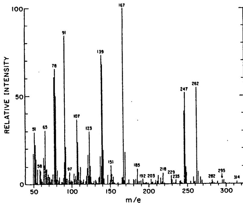
Figure 8. Mass Spectra of Mesurol sulfoxide standard.
