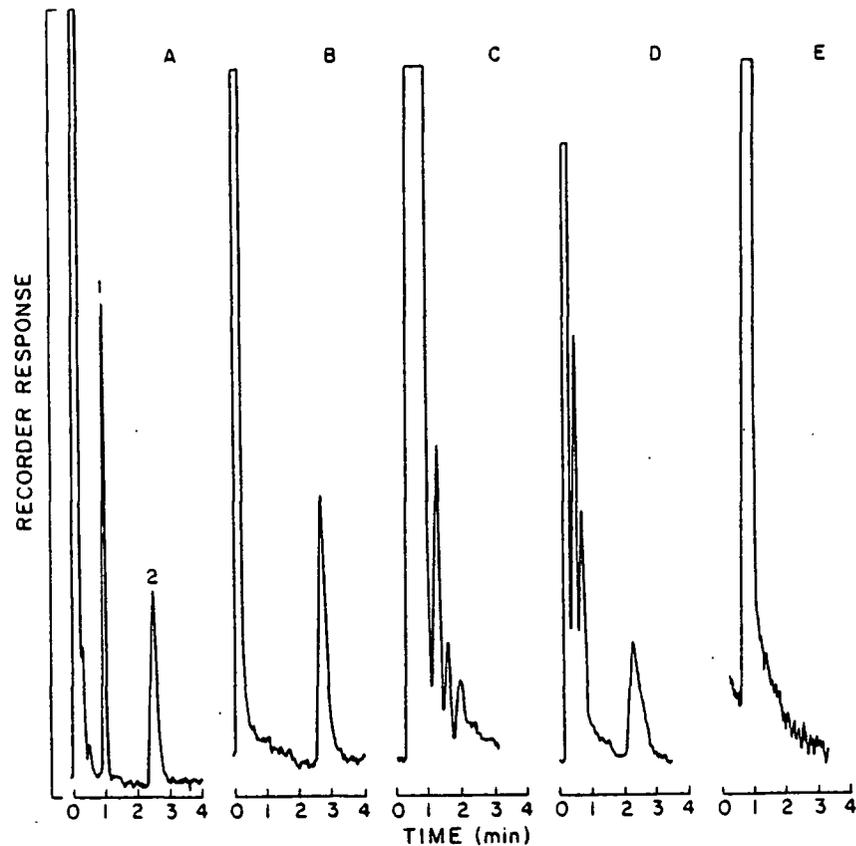
Figure 4. Representative GC chromatograms of Mesurol mesylate derivatives and blanks. Column temperature - 195°C. Attenuation - 8X. (A) Separation of Mesurol sulfide (peak 1) and sulfone (peak 2) Mesylate derivatives (B) Mesurol sulfoxide mesylate. (C) White Riesling juice control, primary. Florisil cut (sulfide and sulfone mesylates). (D) White Riesling juice control, final Florisil cut (sulfoxide mesylate) (E) Pinot Noir juice control, Mesurol total sulfone residue analysis (oxidation).
