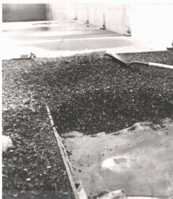
Figure 5.23. Geotextile before failure.
