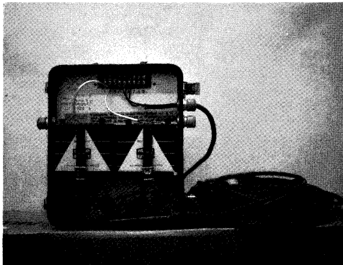
Rear view: door removed; shows power source, rear electronic panel and cable with probe.
