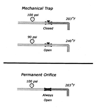
With orifices, each coil consistently has the same heat transfer rate. This results in more consistent drying from top to bottom and from end to end, providing a better quality product and a reduction in drying time per load. Now we can return to the plant level.
