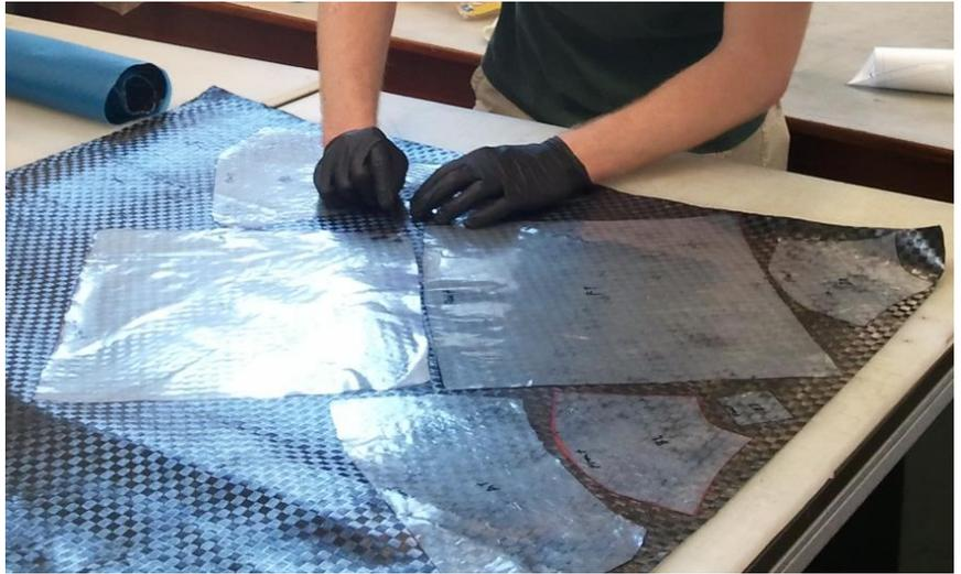
Figure 14: cutting carbon fiber
