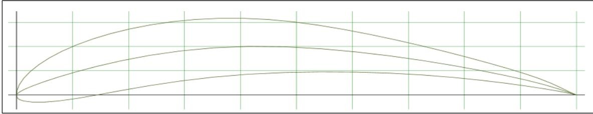
Figure 8: Eppler 423 airfoil [7]
