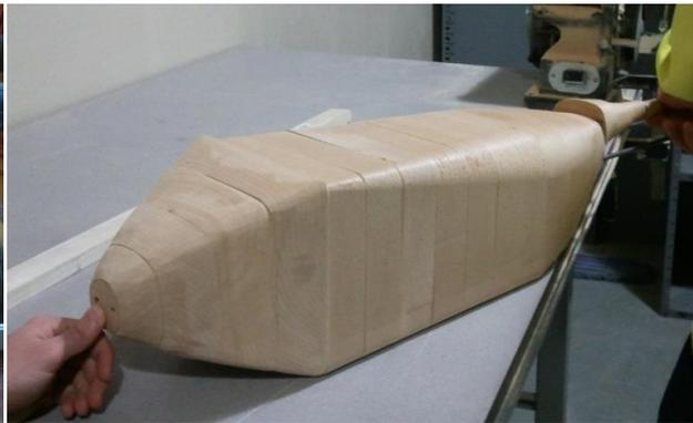
Figure 13: Assembling rough cut mold
