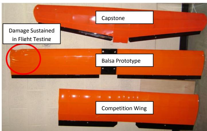
Figure 9: Wing iterations
