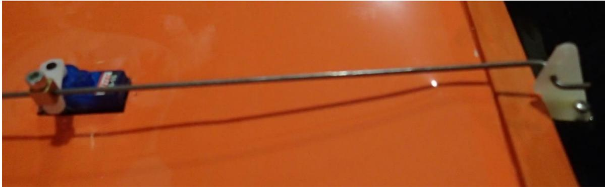
Figure 11: Servo and control rod
