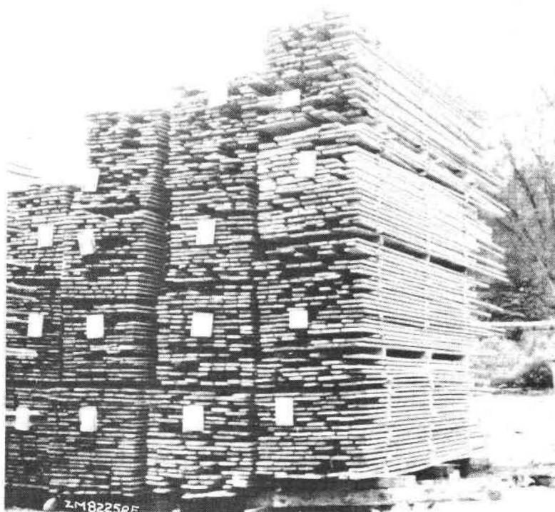
Figure 23. -- Foundations of timbers resting directly on the ground do not provide adequate ground clearance.
