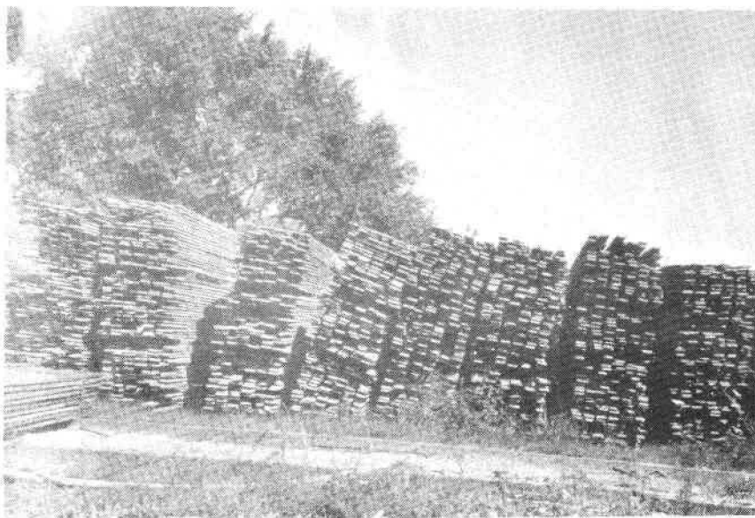
Figure 37. --Several of these package piles have tipped and closed the lateral spaces.
