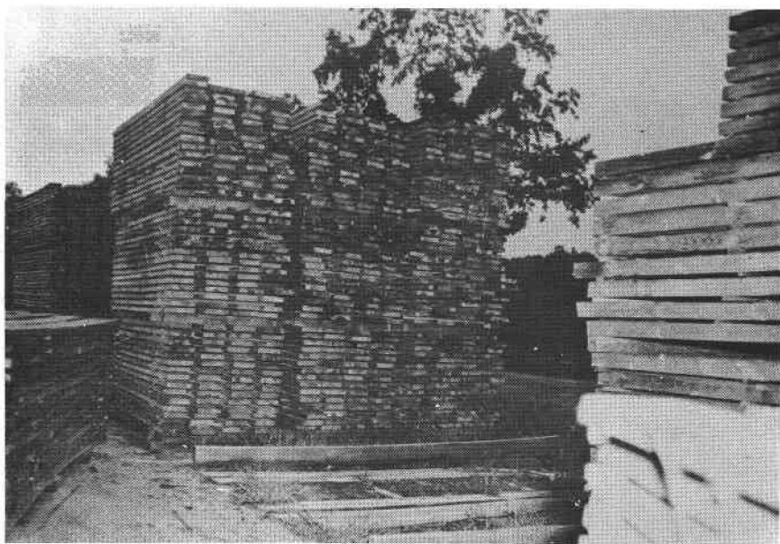
Figure 17. -- The ground clearance in this row of package piles is inadequate, because the foundation consists merely of two timbers resting directly on the ground.
