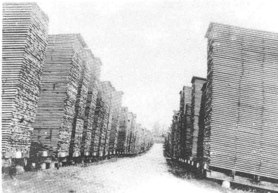
Figure 13. --A main alley in a yard of hand-stacked piles. The freedom from vegetation permits the maximum movement of air over the yard surface and beneath the piles.
