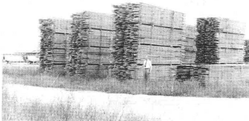
Figure 32. --Since the lumber in this yard is destined for a cross-circulation kiln, the boards are edge-piled in packages 4 feet high and 7 feet wide, with a 1-foot-wide central chimney. The distance between the piles is 8 feet, and the distance between the rows of piles is 12 feet.
