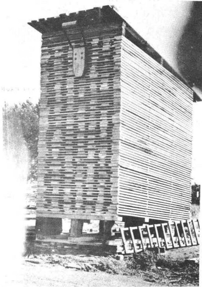
Figure 47. --The front of the double-layered board roof of this hand-stacked pile of hardwood lumber projects about 2 feet beyond the pile and is elevated to increase the pitch of the roof over that of the sloped pile.
