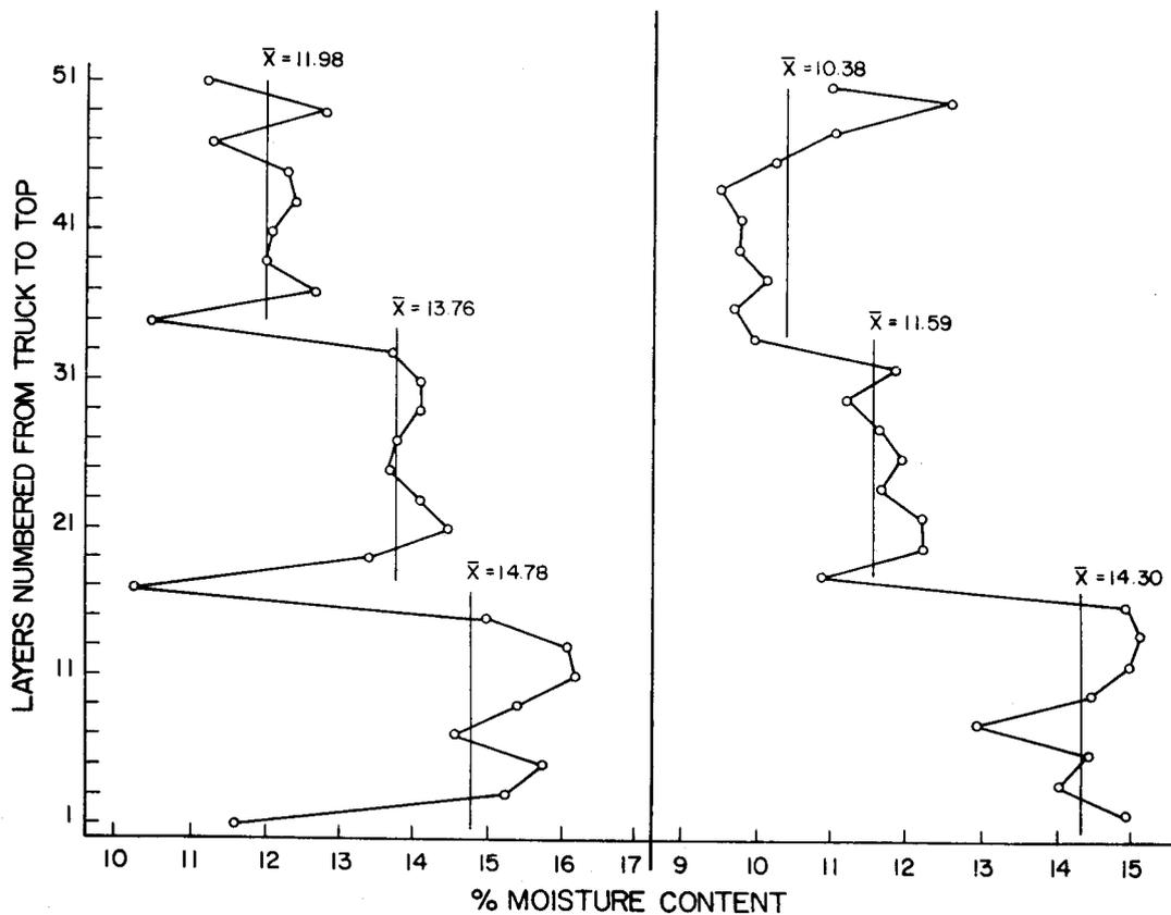
Figure 3. Distribution of final MC as a function of height within the kiln. The 4 x 4 bolsters were located at levels 17 and 35.
