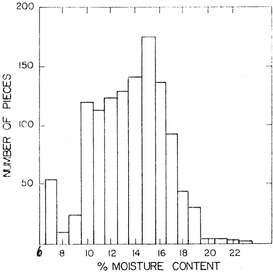
Figure 4. Distribution of final MC for an entire kiln load.
