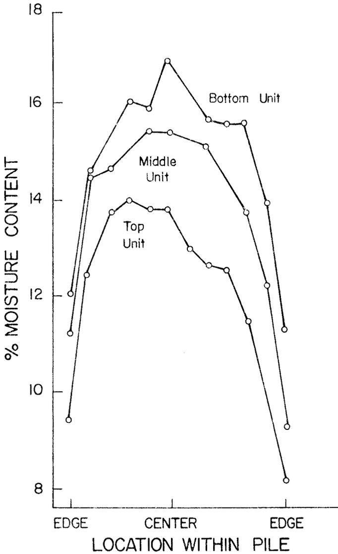
Figure 2. Distribution of final MC within a pile of lumber, for three different heights within the kiln.
