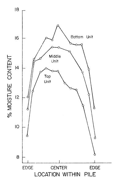
Figure 2. Distribution of final MC within a pile of lumber, for three different heights within the kiln.
