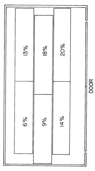
Figure 1. Distribution of final MC within a kiln with poor heat distribution and poor circulation (top view).
