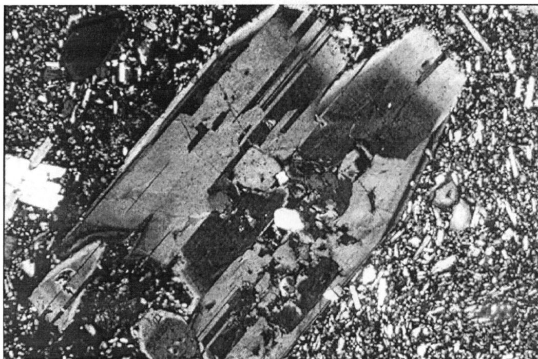
Figure 4.4: Photomicrograph of a Marshall Butte pyroxene. Note the complex sector and oscillatory zoning present. Photo taken at 10x power with polars crossed.
