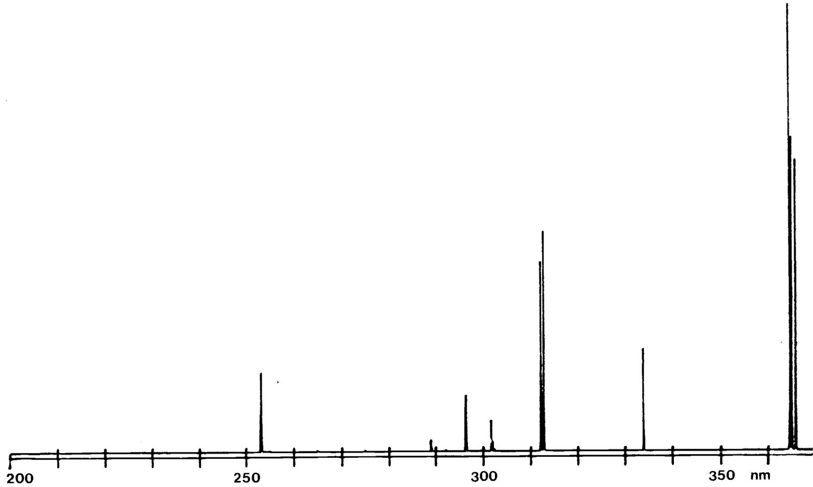
200 nm (no response below about 200 nm). The results are shown in Figure 19. It can be seen from this lamp output spectrum that there is no UV output below 254 nm.
