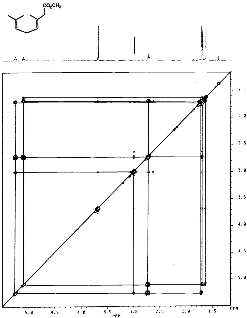
Figure 10.  $^1\text{H}$ ,  $^{13}\text{C}$ -HETCOR Spectrum of Methyl (3Z)-3,7-Dimethyl-3,6-octadienoate, 100.
