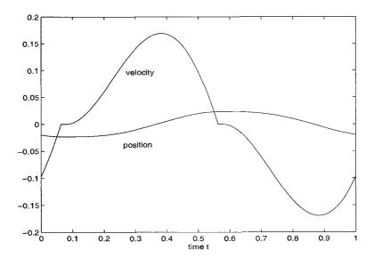
Figure 6. Graph of a periodic solution of the forced dry friction equation (3.5.8)
