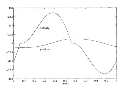
Figure 2. Graph of a periodic solution of the forced dry friction equation (3.5.3)
