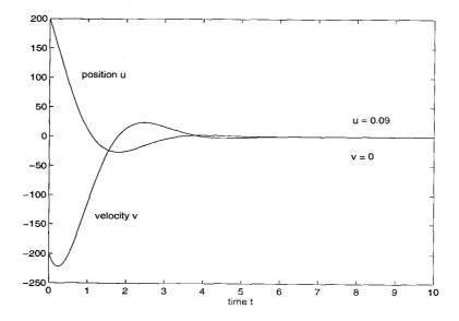
Figure 1. Graph of a solution of the unforced dry friction equation (1.3.3)
