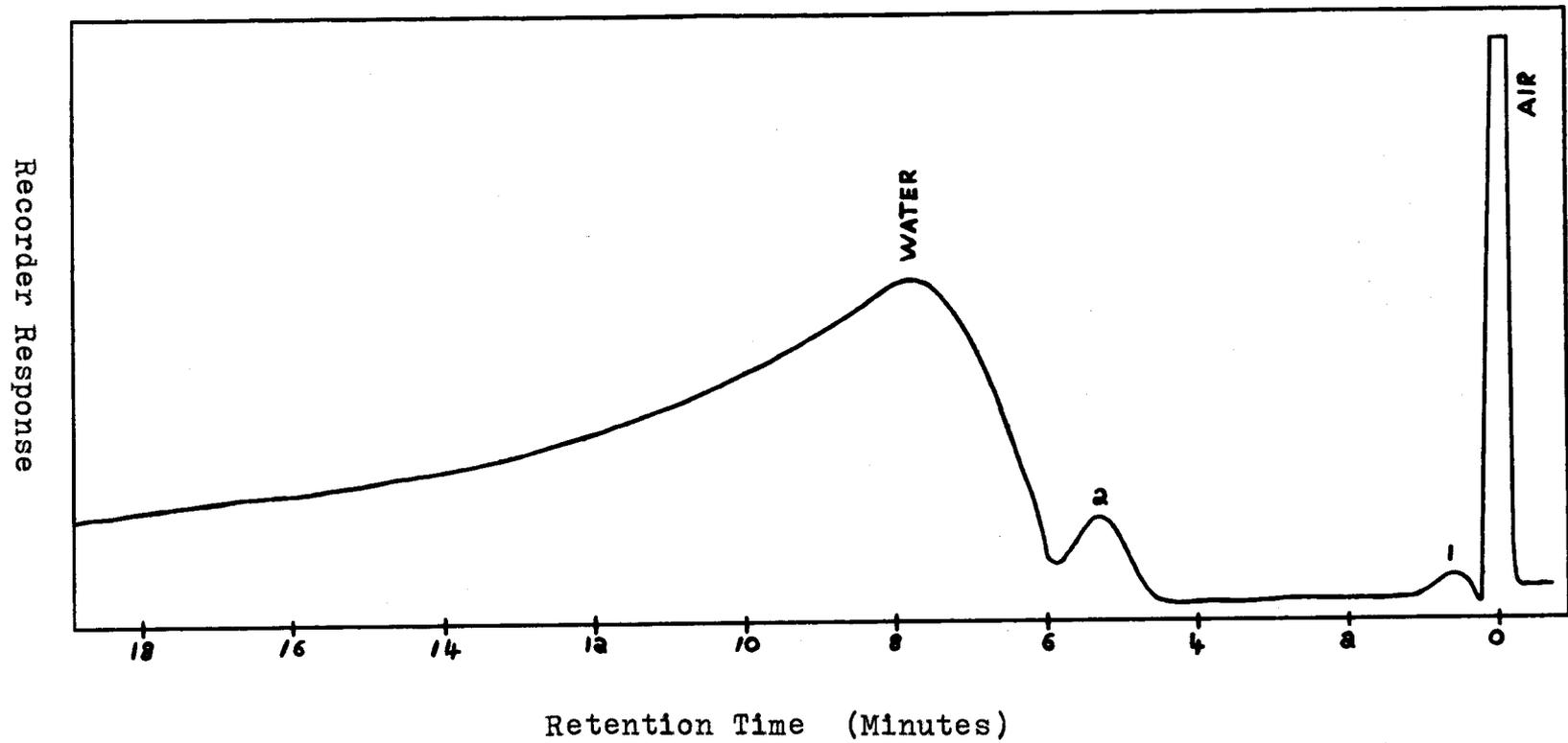
In the second chromatogram shown in Figure 3(b), water presented difficulty since it gave severe tailing. Thus, masking any components that might have been eluted from the column following shortly after the water peak. Probably the best practical solution to this problem would be the use of some method by which the water could be removed prior to analysis without losing any of the sought-for components.
