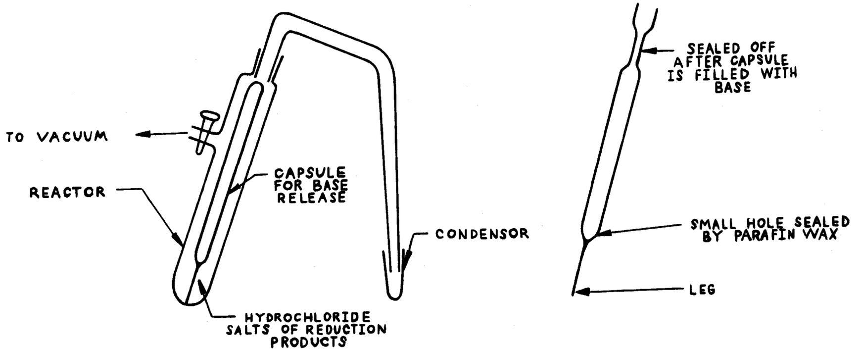
evacuated. As pressure diminished, the air in the capillary blew out the paraffin plug allowing the potassium hydroxide solution out of the capillary.
