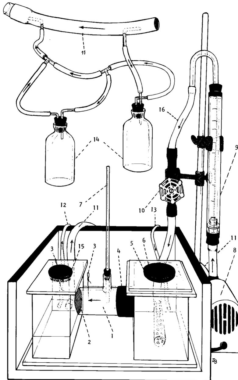
Fig. 3. Tunnel respirometer used for determining the oxygen consumption of unfed and fed fish.
