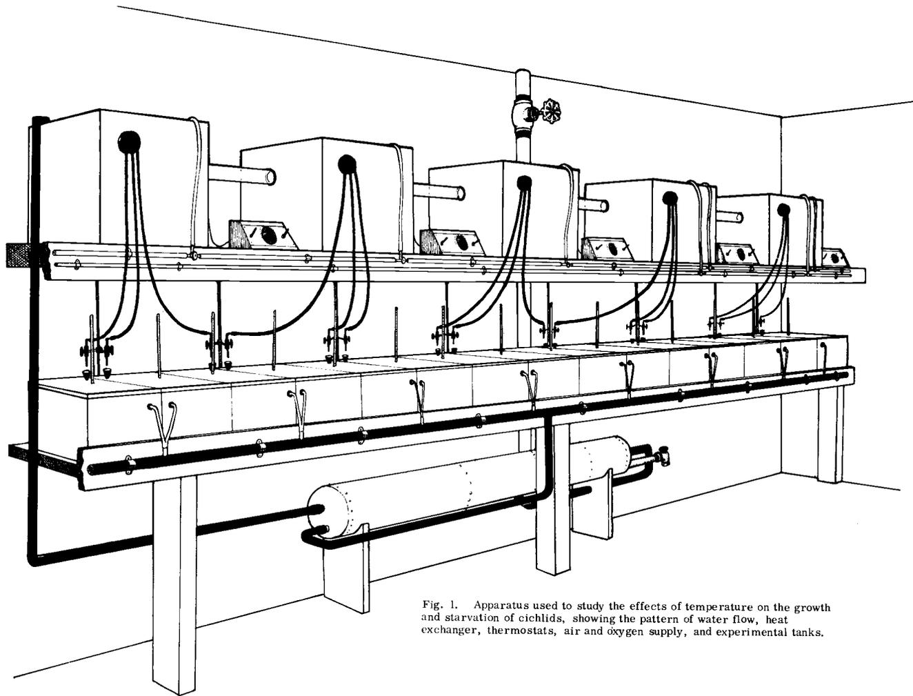
Fig. 1. Apparatus used to study the effects of temperature on the growth and starvation of cichlids, showing the pattern of water flow, heat exchanger, thermostats, air and oxygen supply, and experimental tanks.
