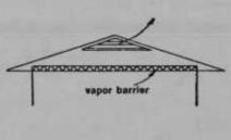
barriers are materials that provide a resistance to the transmission of water vapor. The term used for the rate of water vapor transmission is called *permeance*.
