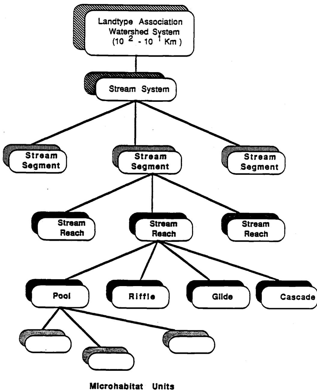
Figure 1. Diagram of a hierarchical watershed model (after Warren and Liss 1983).
