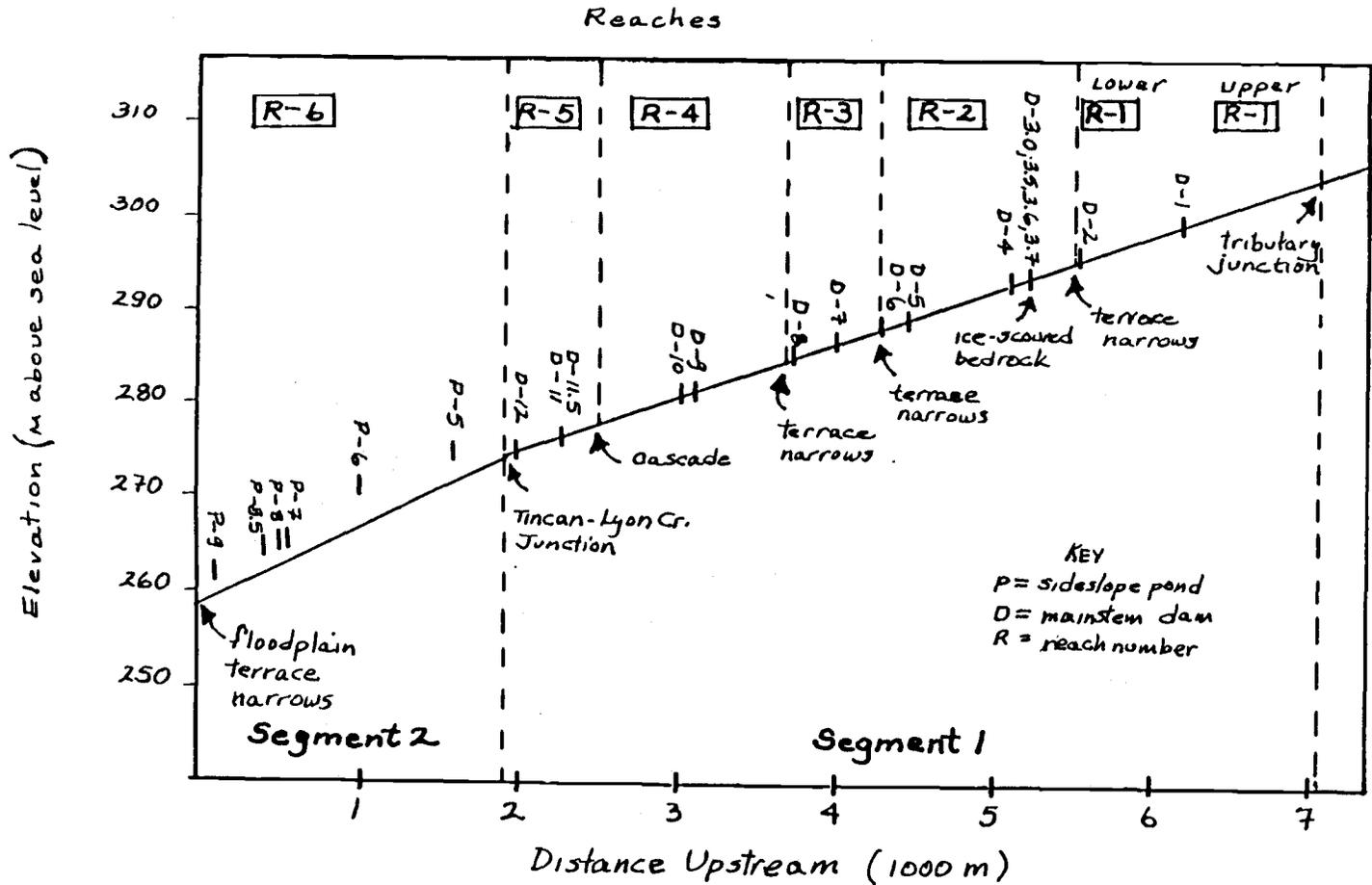
Figure 4. Segment and reach boundaries in relation to beaver dams, channel gradient, and geomorphic features, Upper Granite Creek, 1986.
