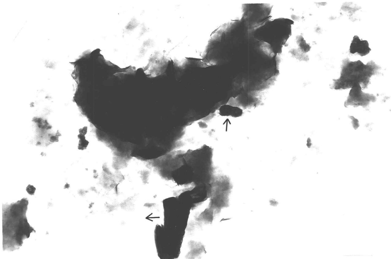
Fig. 5. Transmission electron micrograph of clay particles from unit #1. Hexagonal plates near center (arrow) are probably kaolin, and structure near bottom (arrow) is most likely tubular halloysite. Magnification is 40,000 times.
