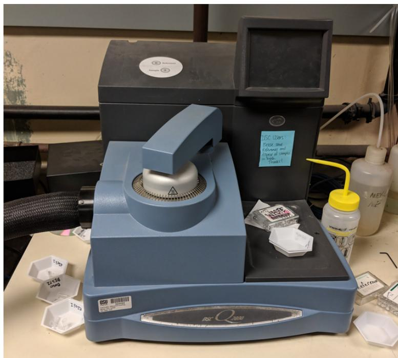
*Figure 4.3: Differential Scanning Calorimetry Q 2000 series used to measure the exothermic and endothermic response of the polymer.*
