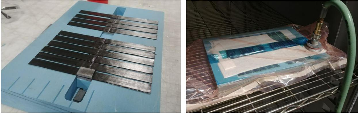
*Figure 4.10: Manufacturing process using a Renshape mold to layup on and vacuum bag to get compaction of the prepreg material.*
