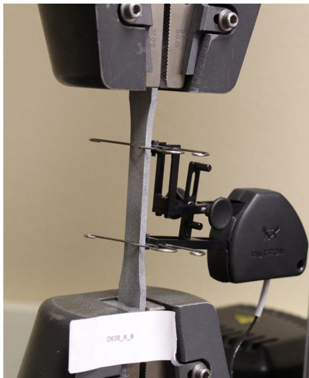
*Figure 4.6: Experimental setup for tensile tests of PA12 samples in the Instron*
