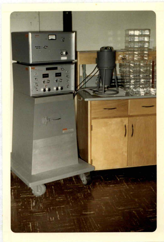
Figure 1. View of counting assembly used in measuring ^{65}\text{Zn} activity in plant samples of Study II.
