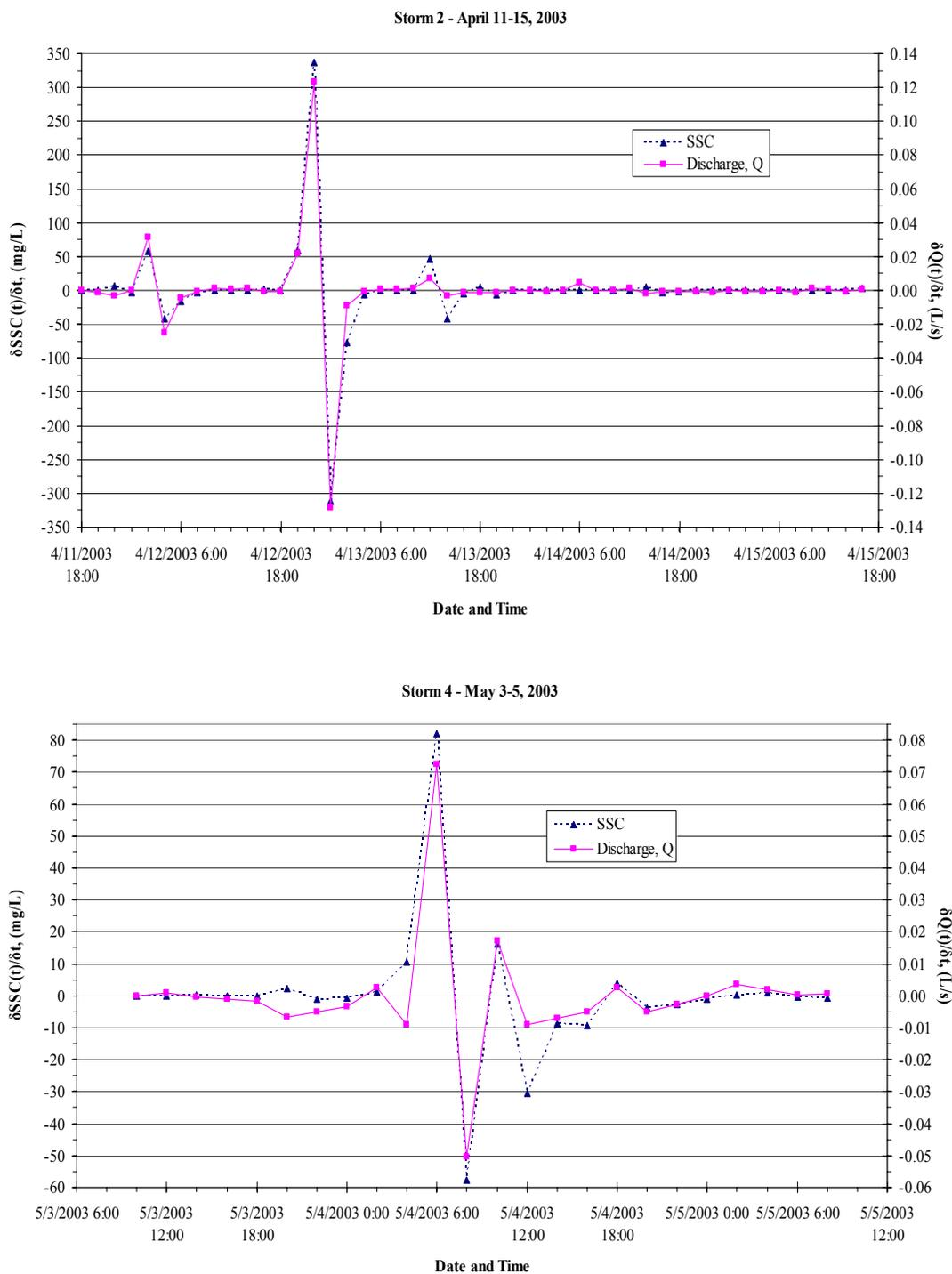
Figure 4.12 First derivatives (i.e. rates of change) of SSC and discharge at culvert 15 for storms 2 and 4.
