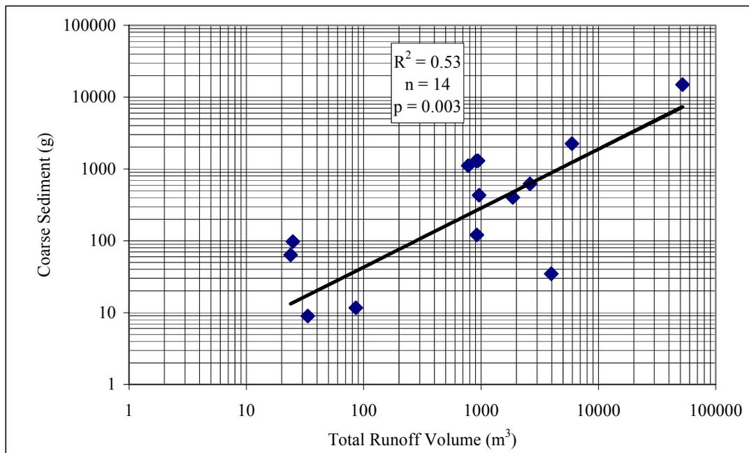
Figure 4. 5 Regression of coarse sediment from geotextile sock on total runoff volume for all culverts.
