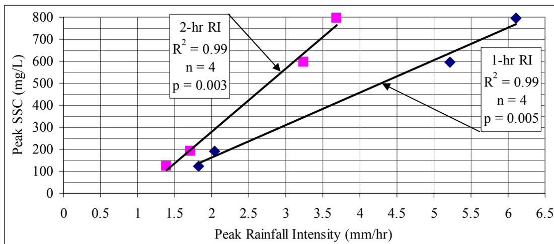
Figure 4.21 Regression of peak suspended sediment concentration on peak 1- and 2-hr rainfall intensity for Storms 1-4 at culvert 15.
