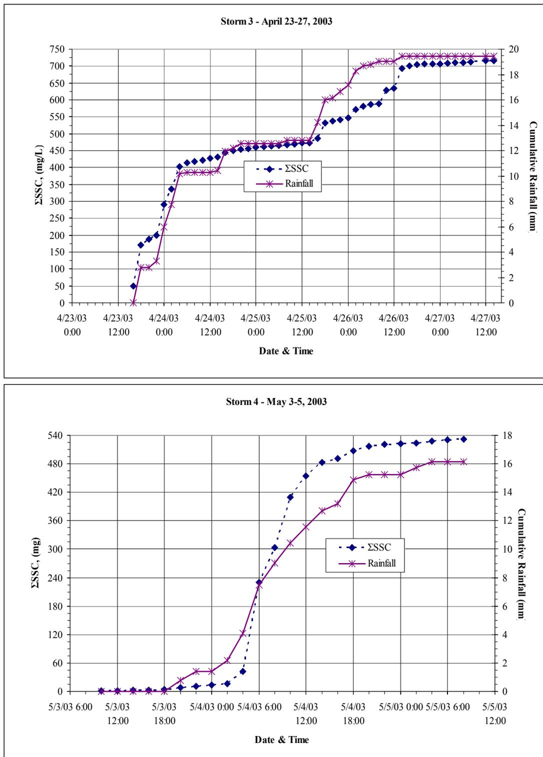
Figure 4. 23  $\Sigma$ SSC and cumulative rainfall at culvert 15 for storms 3 (top) and 4 (bottom).
