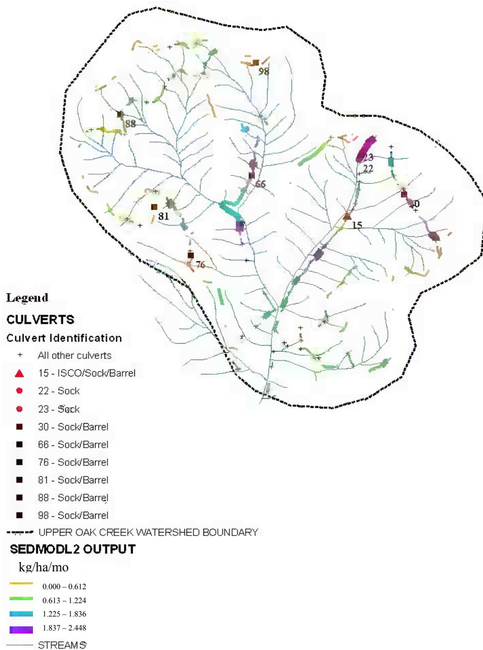
Figure 4.25 Refined SEDMODL2 graphical output with focus on monitored road segments.
