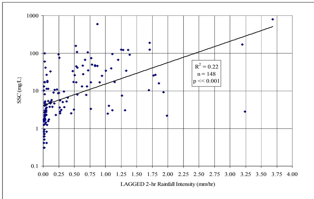
Figure 4.17 Suspended sediment rating curve based on 2-hr rainfall intensity lagged two hours at culvert 15 for storms 1-4. Note: SSC is on log-scale.
