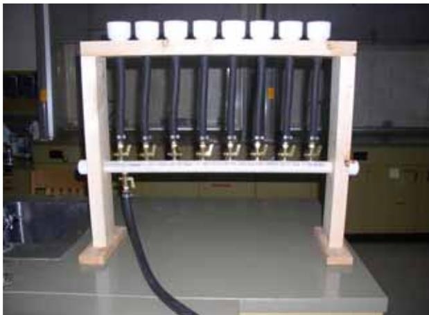
Figure A-1. 1 Vacuum filtration manifold with 8-55mm Buchner funnels.
