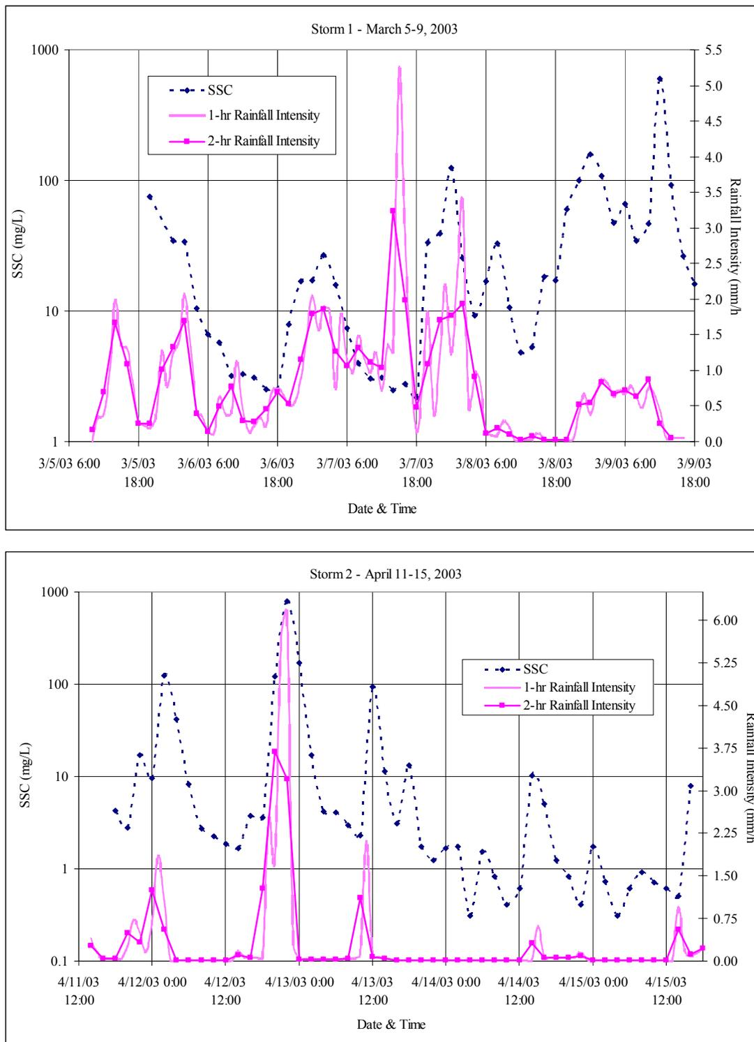
Figure 4. 15 SSC and 1- and 2-hr rainfall intensity at culvert 15 during storms 1 (top) and 2 (bottom). Note: SSC is on log-scale.
