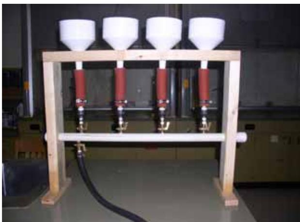
Figure A-1. 2 Vacuum filtration manifold with 4-110mm Buchner funnels.
