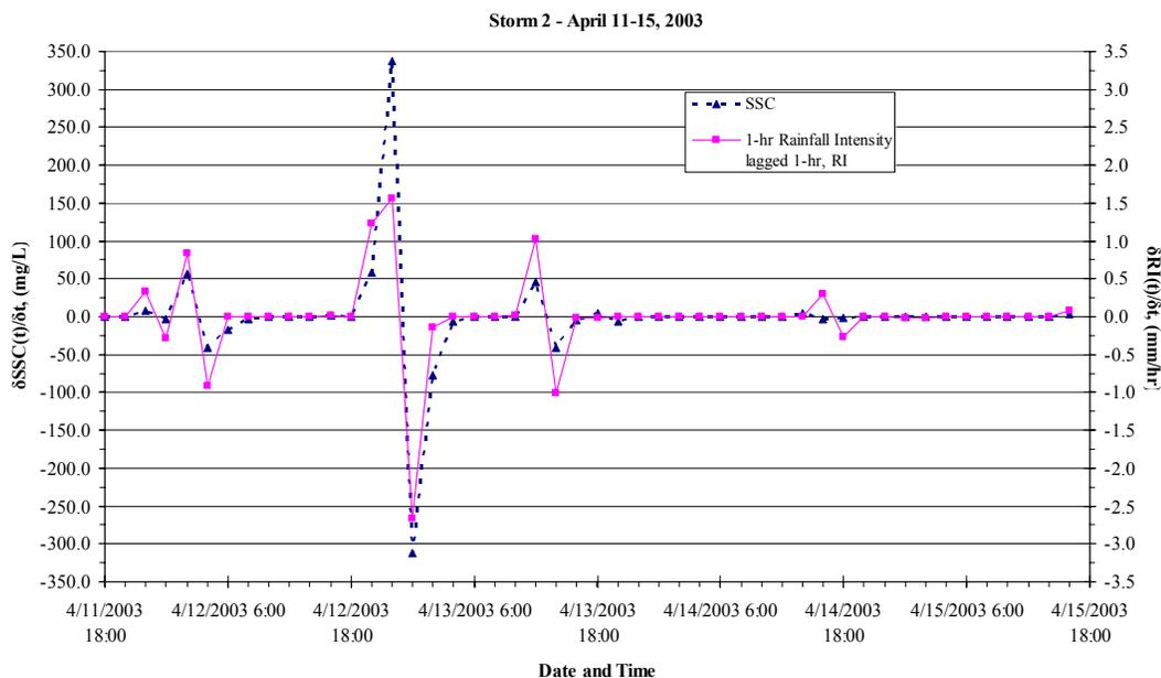
Figure 4.19 First derivatives (i.e. rates of change) of SSC and 1-hr rainfall intensity lagged one hour at culvert 15 for storm 2.
