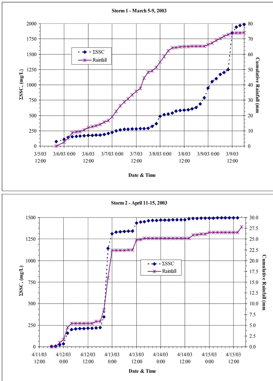
Figure 4. 22  $\Sigma$ SSC and cumulative rainfall at culvert 15 for storms 1 (top) and 2 (bottom).
