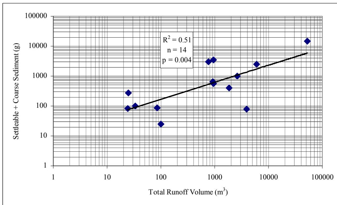
Figure 4.6 Regression of coarse sediment from geotextile sock and settleable sediment from barrels on total runoff volume for all culverts.
