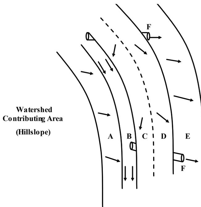
Figure 4. 1 Plan view of a study road segment with associated terminology (adapted from Marbet, 2003). Arrows indicate direction of surface runoff.
