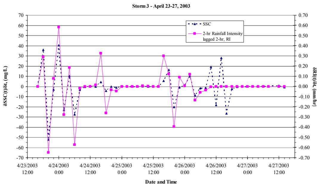
Figure 4.20 First derivatives (i.e. rates of change) of SSC and 2-hr rainfall intensity lagged two hours at culvert 15 for storm 3.
