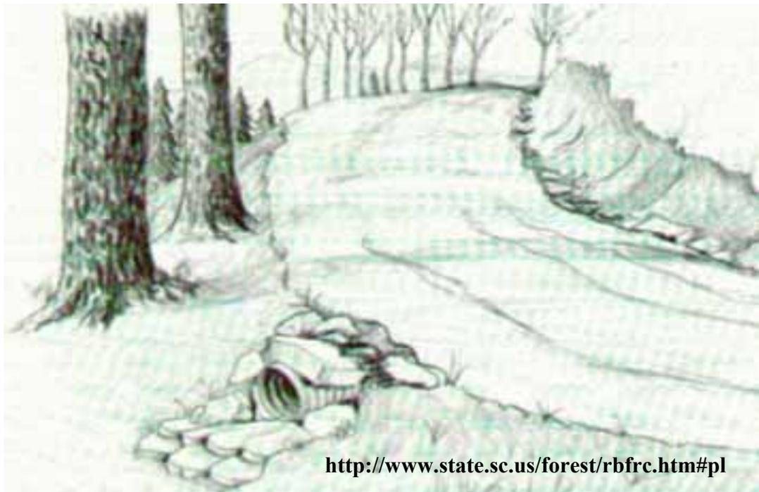
Figure 3. 2 Illustration of cross-drain culvert.
