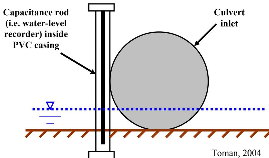
Figure 3. 4 Illustration of capacitance rod installation to measure depth of water entering culvert.
