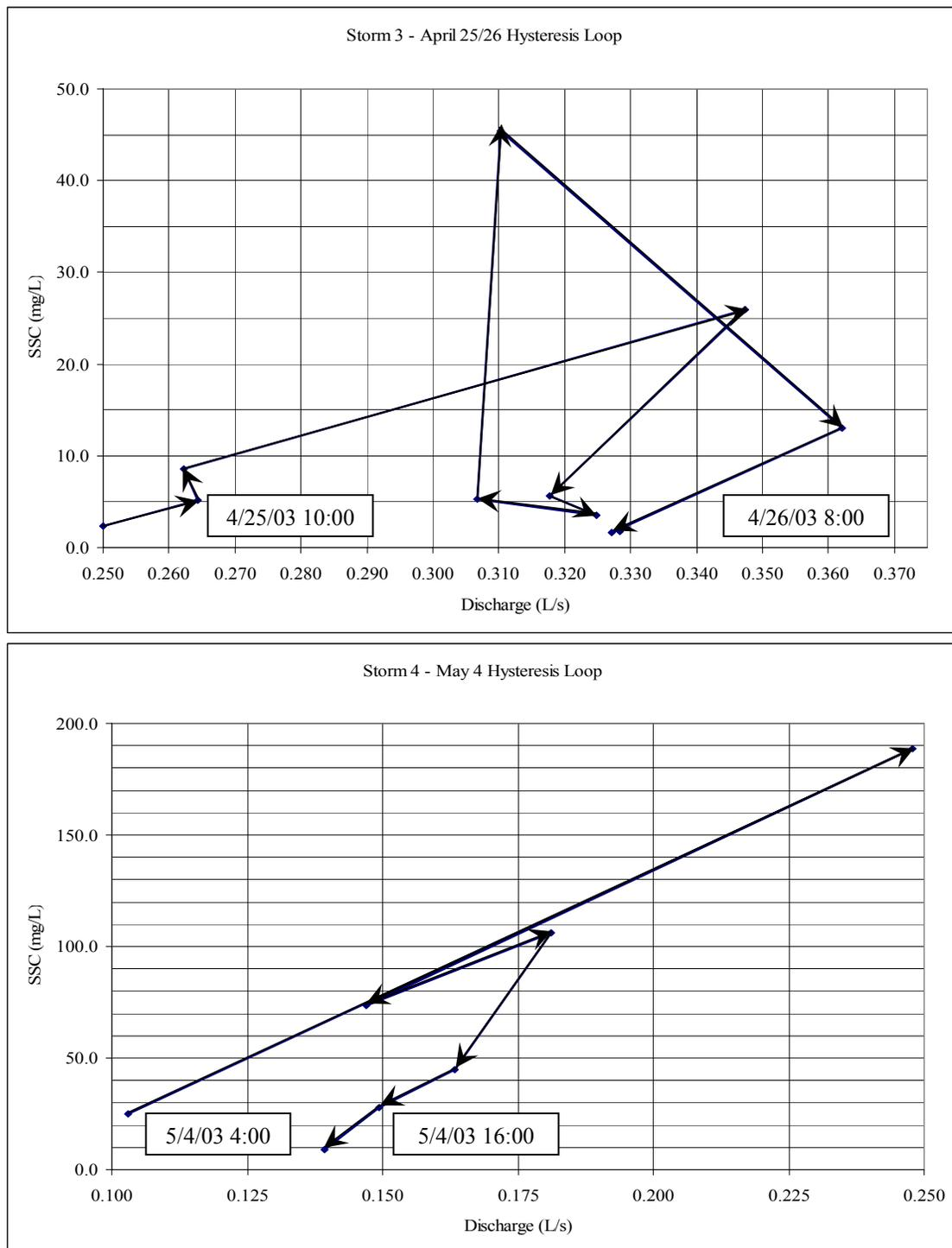
Figure 4. 11 Hysteresis loops for select phases of hydrograph for storms 3 (top) and 4 (bottom) at culvert 15. Arrows indicate progression through time. Boxes containing date and time indicate start and finish of hysteresis loop.
