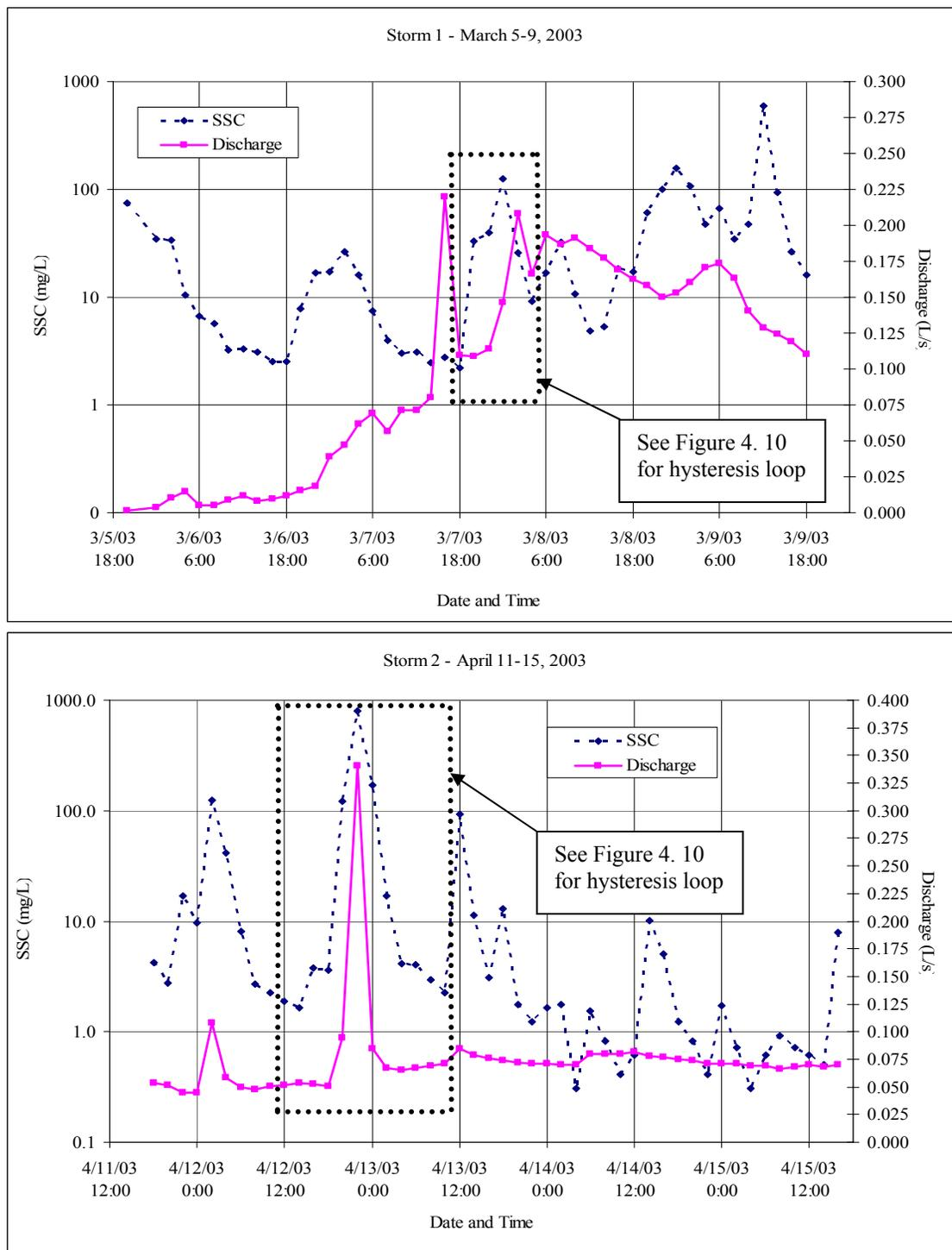
Figure 4. 7 Discharge hydrographs and suspended sediment concentration at culvert #15 for storms 1(top) and 2 (bottom). Dashed boxes indicate sequences of SSC and discharge used to develop the hysteresis plots shown in Figure 4. 10. Note: SSC is on log-scale.
