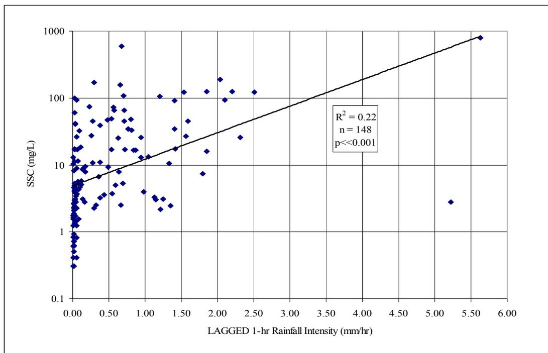
Figure 4.18 Suspended sediment rating curve based on 1-hr rainfall intensity lagged one hour at culvert 15 for storms 1-4. Note: SSC is on log-scale.
