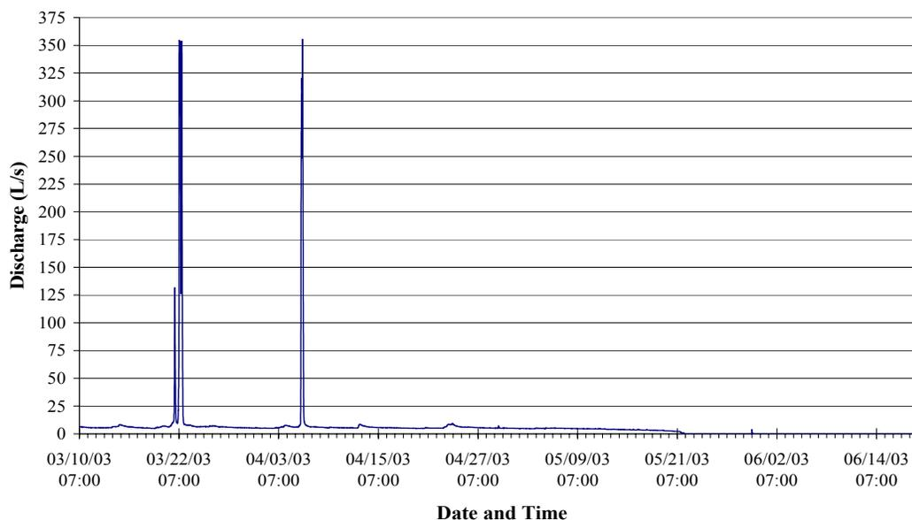
Figure 4. 2 Culvert 23 hydrograph from 03/10/03 through 06/19/03 with peak discharges occurring on 03/22 and 04/06. Note the absence of extended falling limbs as well as the absence of elevated discharge depth after the peak discharges.
