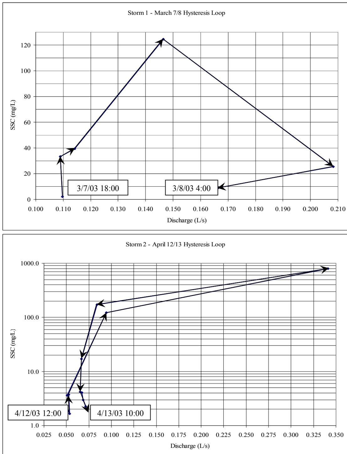
Figure 4. 10 Hysteresis loops for select phases of hydrograph for storms 1 (top) and 2 (bottom) at culvert 15. Arrows indicate progression through time. Boxes containing date and time indicate start and finish of hysteresis loop.
