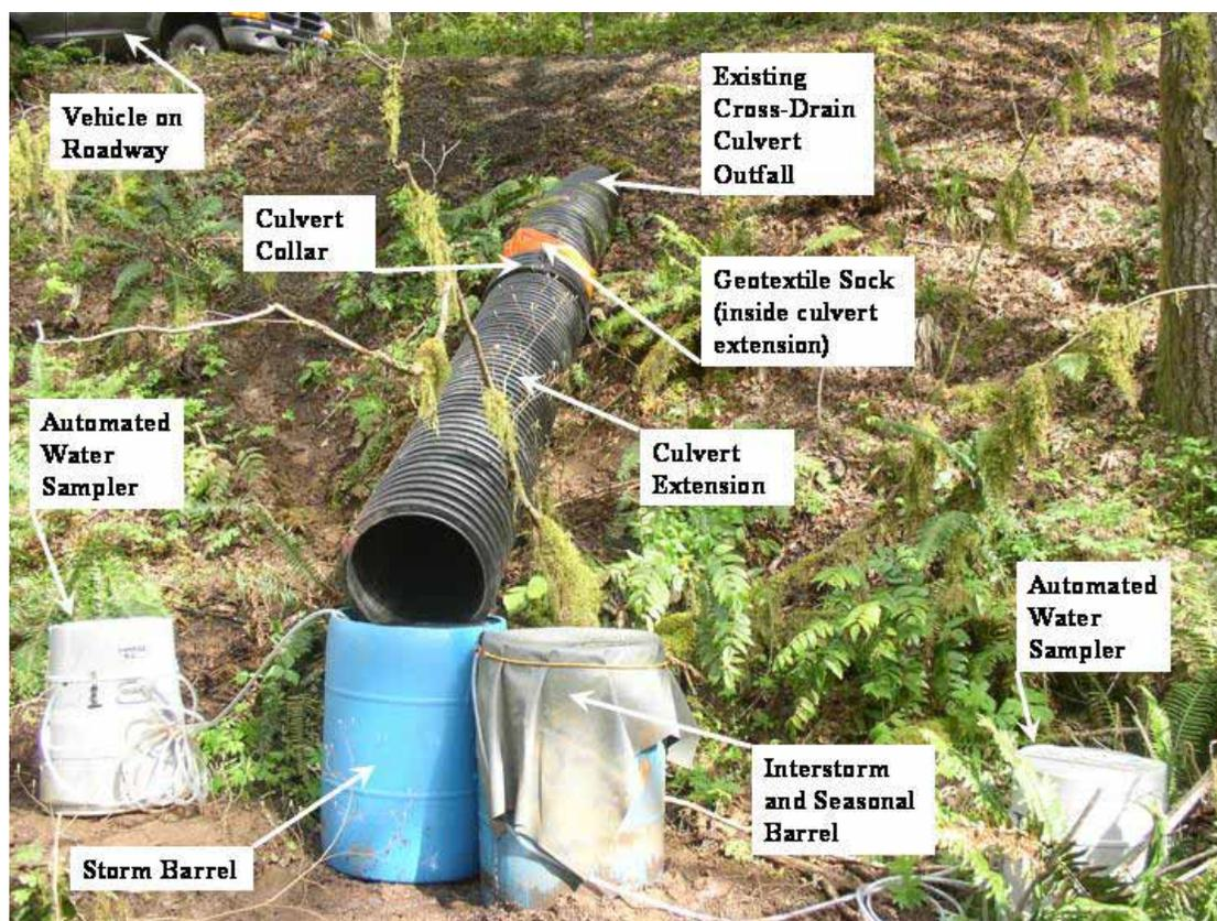
Figure 3. 7 Complete sediment trap used at culvert 15.
