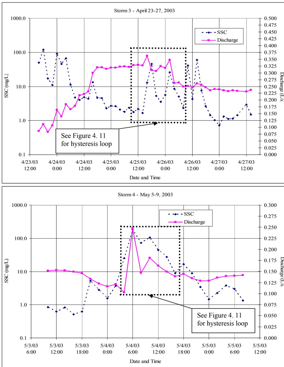
Figure 4. 8 Discharge hydrographs and suspended sediment concentration at culvert #15 for storms 3 (top) and 4 (bottom). Dashed boxes indicate sequences of SSC and discharge used to develop the hysteresis plots shown in Figure 4. 11. Note: SSC is on log-scale.
