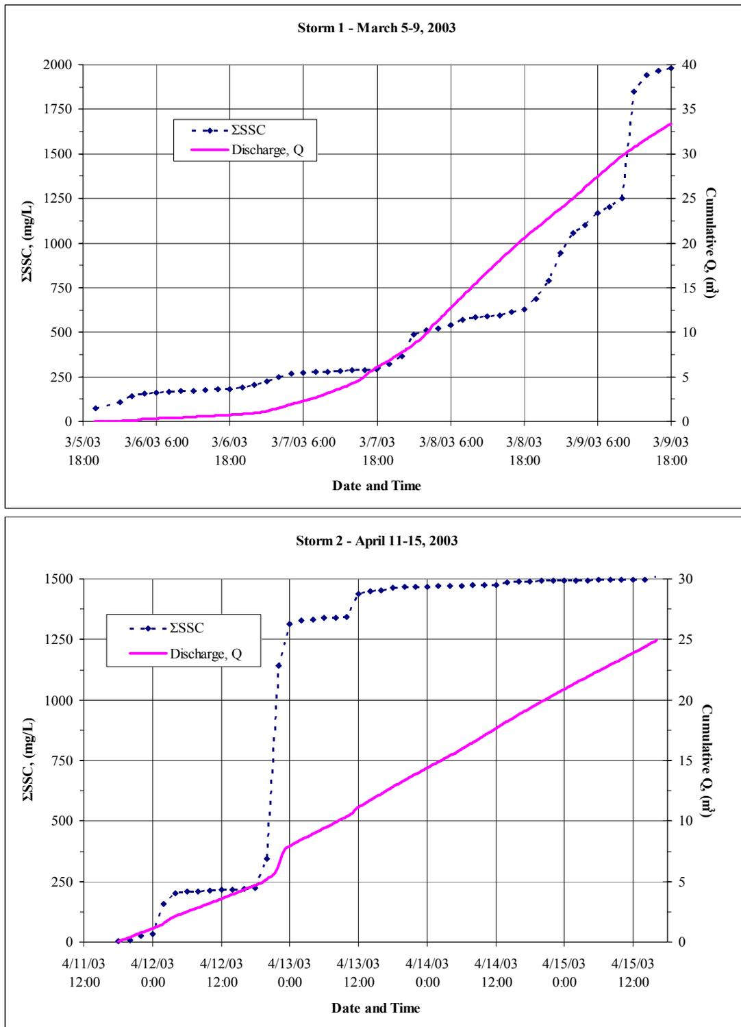
Figure 4. 13 ΣSSC and cumulative discharge at culvert 15 during storms 1 (top) and 2 (bottom).
