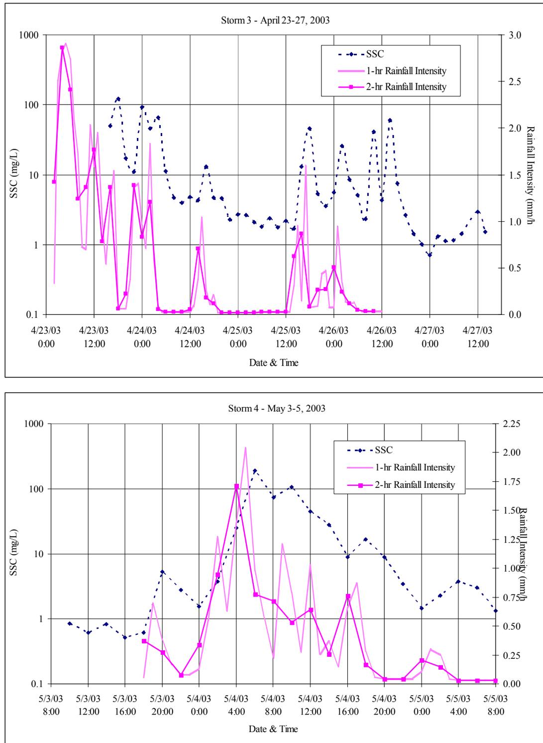
Figure 4. 16 SSC and 1- and 2-hr rainfall intensity at culvert 15 during storms 3 (top) and 4 (bottom). Note: SSC is on log-scale.
