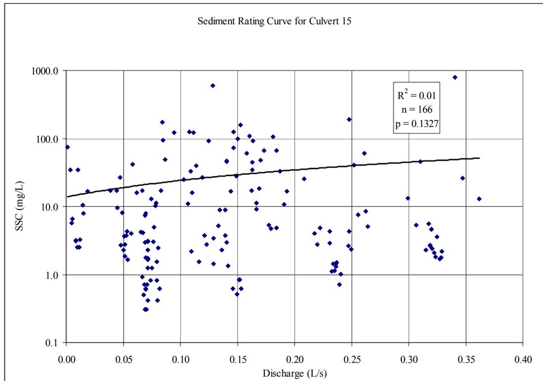
Figure 4.9 Sediment rating curve for culvert 15. Data points from storms 1-4.
