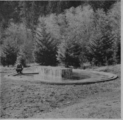
Specially designed outdoor ponds will enable scientists to study fish at different oxygen concentrations under conditions closely akin to nature.
