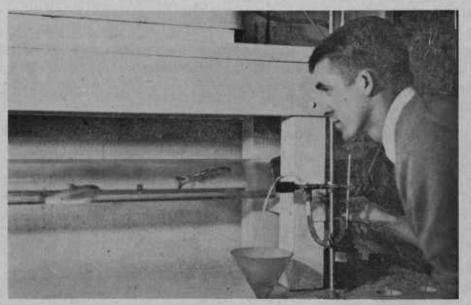
OSU researcher D. L. Shumway checks fish swimming ability in water of varying oxygen concentration which is pumped through tube at varying velocity.
