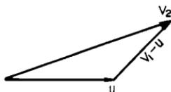
$$v_2 = u + (v_1 - u)$$
