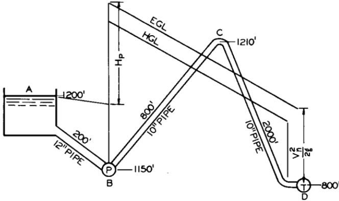
Theory: The problem consists of recognizing and evaluating energy losses in pipe and nozzle, and energy relationships between static, velocity, and pressure heads.
