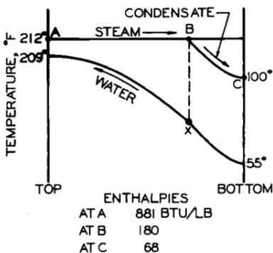
From A to B the steam will be considered at 212°F, while from B to C the temperature of the condensate will drop from 212°F to 100°F.
