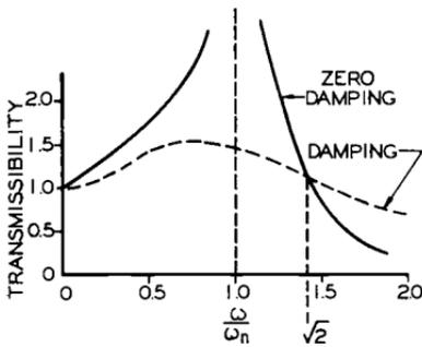
a) If the transmitted force is to be small, the natural frequency of the support must be very low compared to the frequency of the impressed force (as when mounting a machine on springs).
