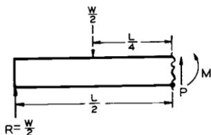
Note that at the cut section there must be a vertical force up (shear), as well as an upward moment  $M$ . These represent internal stresses which, after cutting, become external to the free body being considered.
