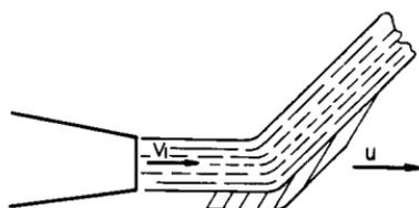
moves across it per unit of time, with a velocity relative to the vane of  $(v - u)$ . The final absolute velocity of the fluid must first be found.
