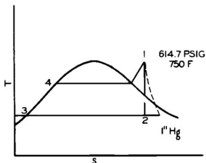
Condition 2 has the same entropy, and is vertically below 1 on the diagram.
