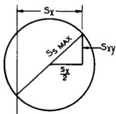
subjected both to normal stresses due to bending and to shear stresses due to torsion. Since failure will be in shear, the maximum shear stress resulting from the combined bending and torsion must be determined. Also, since the shaft is rotating, some concern must be given to fatigue in bending.
