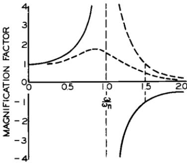
Under conditions of forced vibration, such as that due to "out-of-balance," the amplitude of vibration may become excessive at one or more "critical" speeds. These critical speeds correspond to one of the natural frequencies of the supporting structure. Amplitude or vibration can be determined from the equation
