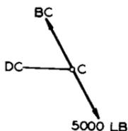
Pin C: Link DC must have zero force because there would be no way to react the component perpendicular to BC.
