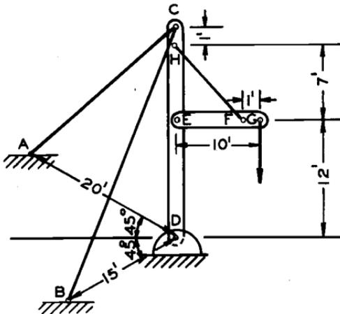
Solution: Since the cables are two-force body members, forces must act along the length of the cables. Draw a free-body diagram of the mast and boom with external forces shown. Cable tensions are shown broken down into their x, y, and z components.
