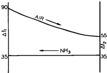
where  $\Delta t_m$  is the mean temperature difference. Here, the mean  $\Delta t$  must be determined as the log mean temperature difference.
