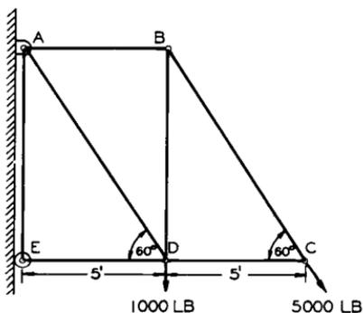
Theory: In truss problems it is assumed all loads are applied at a pin and each member is free to turn at the pin. This makes all members two-force body members, either in tension or compression.
