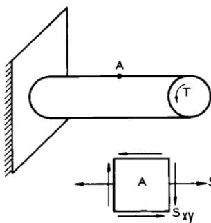
Looking down on point A, the stress condition on a small element would appear as in the sketch below the shaft. Using Mohr's circle it is apparent that
