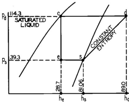
from c to e, and some of the liquid vaporizes. The remainder vaporizes in the evaporator e to s, where heat is removed from the refrigerated space.
