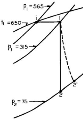
Since back pressure on the nozzle (75 psia) is less than critical pressure ( $p_c = 0.55 p_2 = 173$  psia), flow through the nozzle is independent of back pressure and may be calculated using Grashof's formula (Marks, p. 335).
