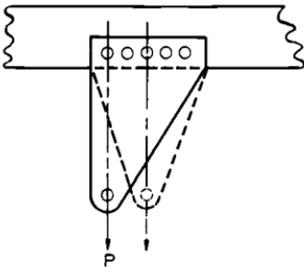
Theory: All problems of eccentric loading are treated in the same manner. The existing force system is replaced by an equivalent force system which can be more easily handled.
