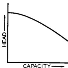
Actual flow for a pump operated at a speed of 1160 rpm will vary with the head in a manner similar to the curve shown. It is apparent that if the pump is operated against a head of 55 feet of water instead of 57 feet, the capacity will be somewhat greater than 398 gpm.
