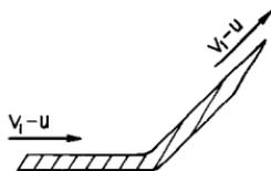
The absolute velocity of the fluid leaving the vane is equal to absolute velocity of vane plus, vectorially, the relative velocity of the fluid with respect to the vane.
