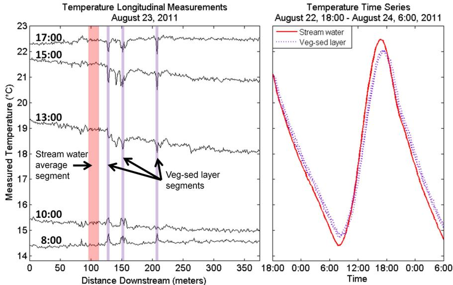
**Figure 2.** DTS stream temperature measurements taken at 08:00, 10:00, 13:00, 15:00 and 17:00 PST along 375 m of the Middle Fork John Day River are shown on the left, with segments that intersected vegetation–sediment layers (centered at 129, 152, and 208 m downstream) highlighted in purple. On the right, these temperature measurements within the layers were plotted temporally with average ambient stream water temperature (distance-averaged temperature from 96 to 116 m downstream).
