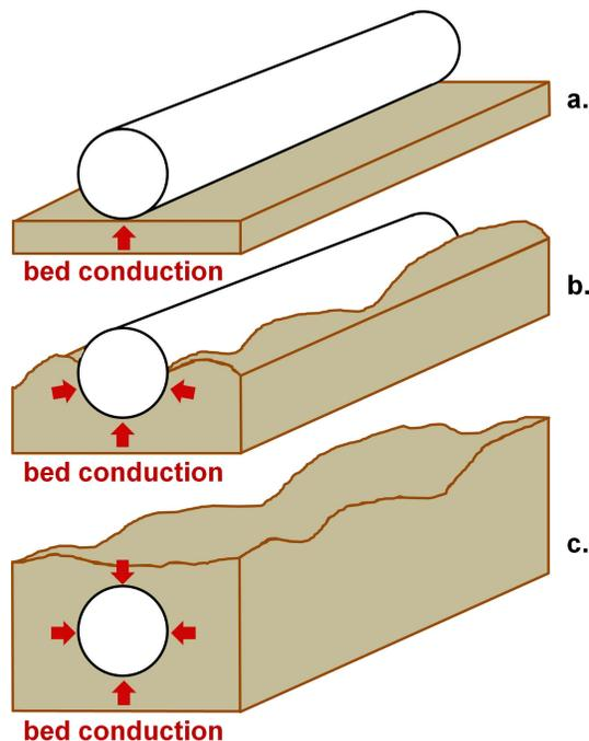
**Figure 1.** The impact of bed conduction on DTS measurements depends on the degree of fiber optic cable burial within bed materials, including **(a)** not buried, **(b)** partially buried, and **(c)** fully buried.
