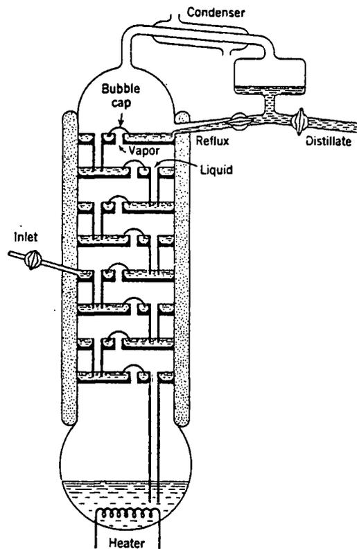
Figure 2. Bubble-cap Fractionating Column
