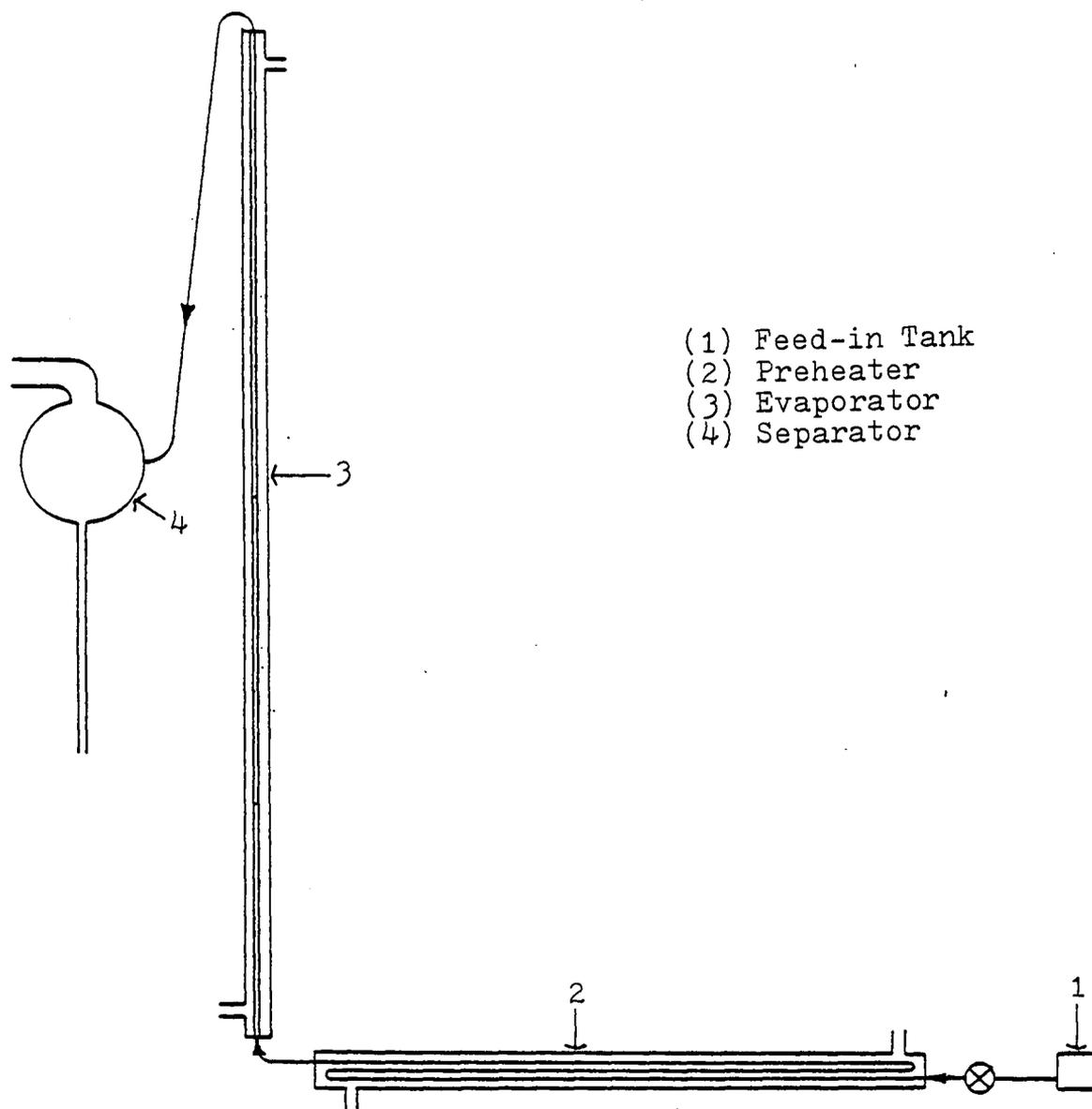
Figure 4. Preheater and Evaporator
