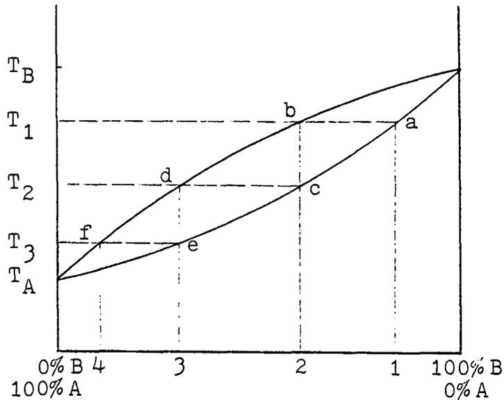
Figure 1. Boiling Point/Composition Diagram
