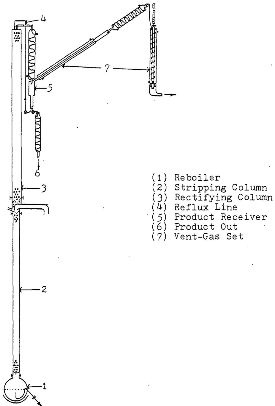
Figure 6. Fractional Distillation System
