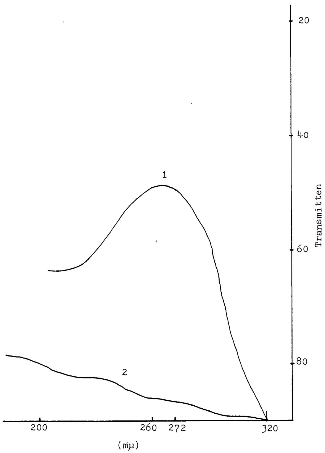
Figure 14. Ultraviolet Spectra of Pear Essence (1) and Reboiler Discharge Water (2)
