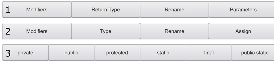
Figure 2.2: The options row is empty until a key is pressed. The top, middle, and bottom images show the appearance for the options row after pressing the “function”, “variable”, and “modifiers” keys respectively.
