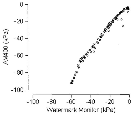
Figure 1. Response of Watermark soil moisture sensors to irrigation events and the termination of irrigation as measured by an AM400 Hansen datalogger (A) and an Irrrometer Watermark Monitor (B). The average readings of the an AM400 Hansen datalogger and an Irrrometer Watermark Monitor are compared over time (C) and over the measured range of soil water potential (D), Malheur Experiment Station, Oregon State University, Ontario, OR, 2003.
