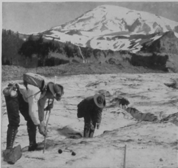
Measuring the Ice Flow in Nisqually Glacier. In 1905 Prof. J. N. Le Conte of Berkeley, Cal., established the fact that this glacier has an average flow, in summer, of 16.2 inches a day. The movement is greater at the center than on the sides, and greater on the convex side of a curve than on the concave side. It thus is a true river, though a slow one. The measurements are taken by running a line from one lateral moraine to the other with a transit, setting stakes across the glacier at short intervals, and ascertaining the advance they make from day to day.
