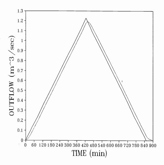
Figure 17. A 50-year storm event inflow and outflow hydrographs for a large-sized (6002  $\mathrm{m}^2$ ) pond in a watershed 10 times large than the pond.
