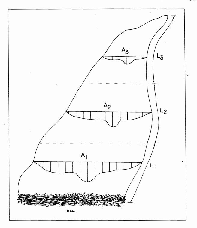
Figure 4. Layout of pond measurements.
