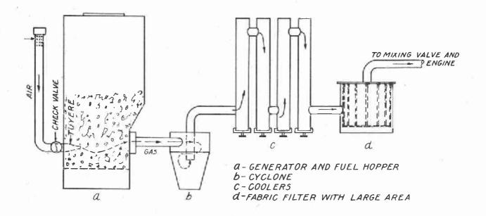
Figure 1.--Schematic drawing showing the principal parts of a charcoal-burning gasogen.
