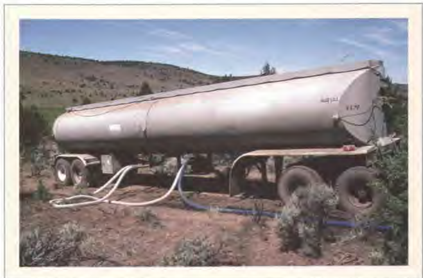
Figure 2. A 9,000-gallon tanker was required to supply water for each simulation run. It took 10 days to complete 16 simulation runs for the field portion of the project.
