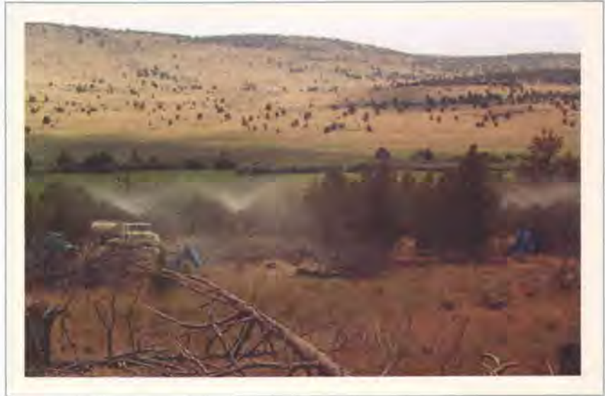
Figure 1. There were eight replications of cut and uncut plots. In every case the uncut plots experienced runoff and erosion. This picture shows the rainfall simulator application on cut (left) and woodland (right) treatments.
