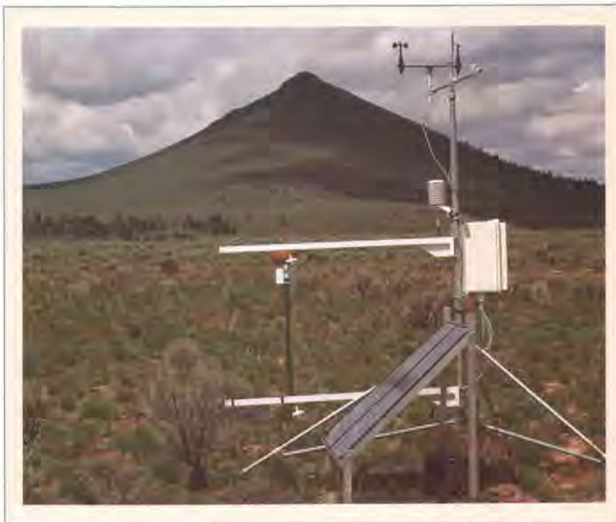
Figure 1. Bowen ratio energy balance instrumentation (Model 023/ \text{CO}_2 , Campbell Scientific, Inc., Logan, Utah, USA)
