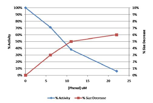
**Figure 1**. The effect of increasing phenol concentration on % activity and % size decrease of *N*. *europaea* cells. An increase in % size decrease corresponds to a decrease in cell size. Increasing phenol concentrations resulted in a decrease in activity and a simultaneous steady decrease in cell size. The data suggests an asymptotic approach to just above 6% decrease in cell size as activity decreases to zero.
