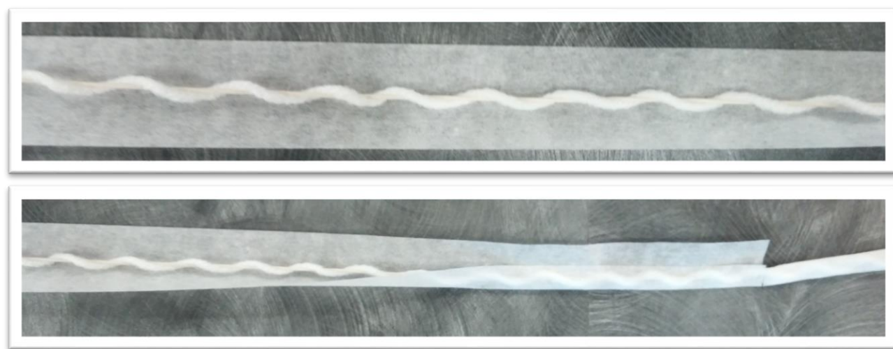
Figure 7 a, b: Figure 7 a shows the initial design of the wet bulb fiber optic cable. The cable was first coiled with a blended cotton and acrylic yarn of medium weight. A similar design, without the addition of the cotton/acrylic yarn was used in the John Day, OR field experiments.
